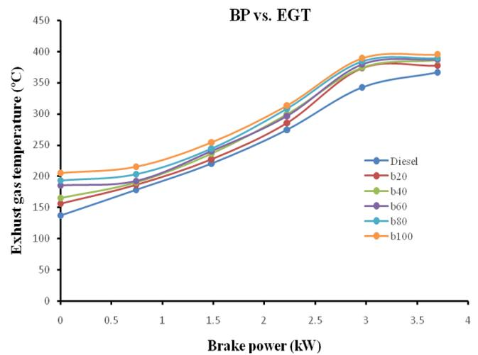
**Figure 7:** Variation on exhaust gas temperature
