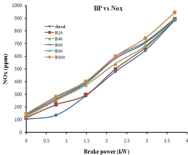
**Figure 6:** Variation on oxides of nitrogen (NOx) emission
