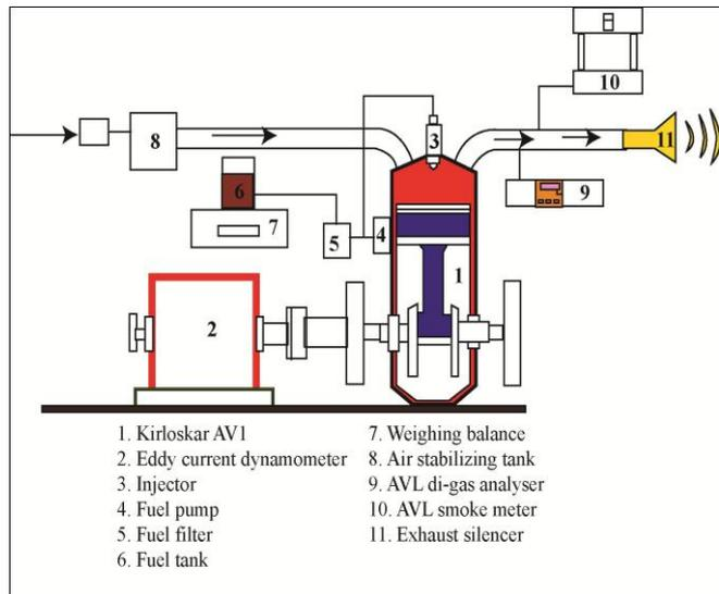
**Figure 1:** Schematic diagram of the experimental engine setup
