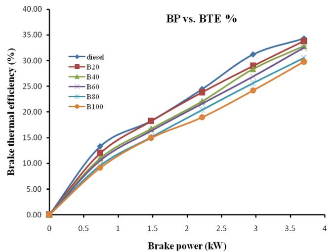
Figure 5: Variation on Brake thermal efficiency
