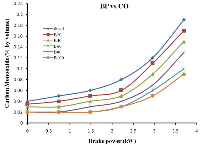
Figure 4: Variation on Carbon monoxide emission
