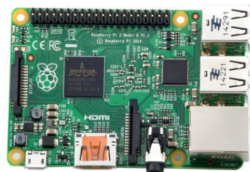
Figure 1: Raspberry Pi 2B [13].
