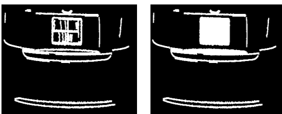
Figure 13: dilation using 4x4 square structure element (left) and filling holes to construct objects (right)
