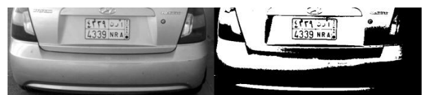
Figure 2: Segmentation process using pixel intensity threshold
