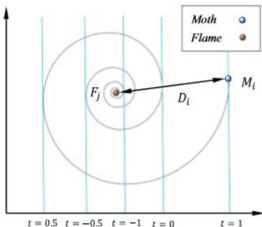
**Figure 3:** Logarithmic spiral, space encompassing the flame & considering the different 't' position on the curvature [29]
