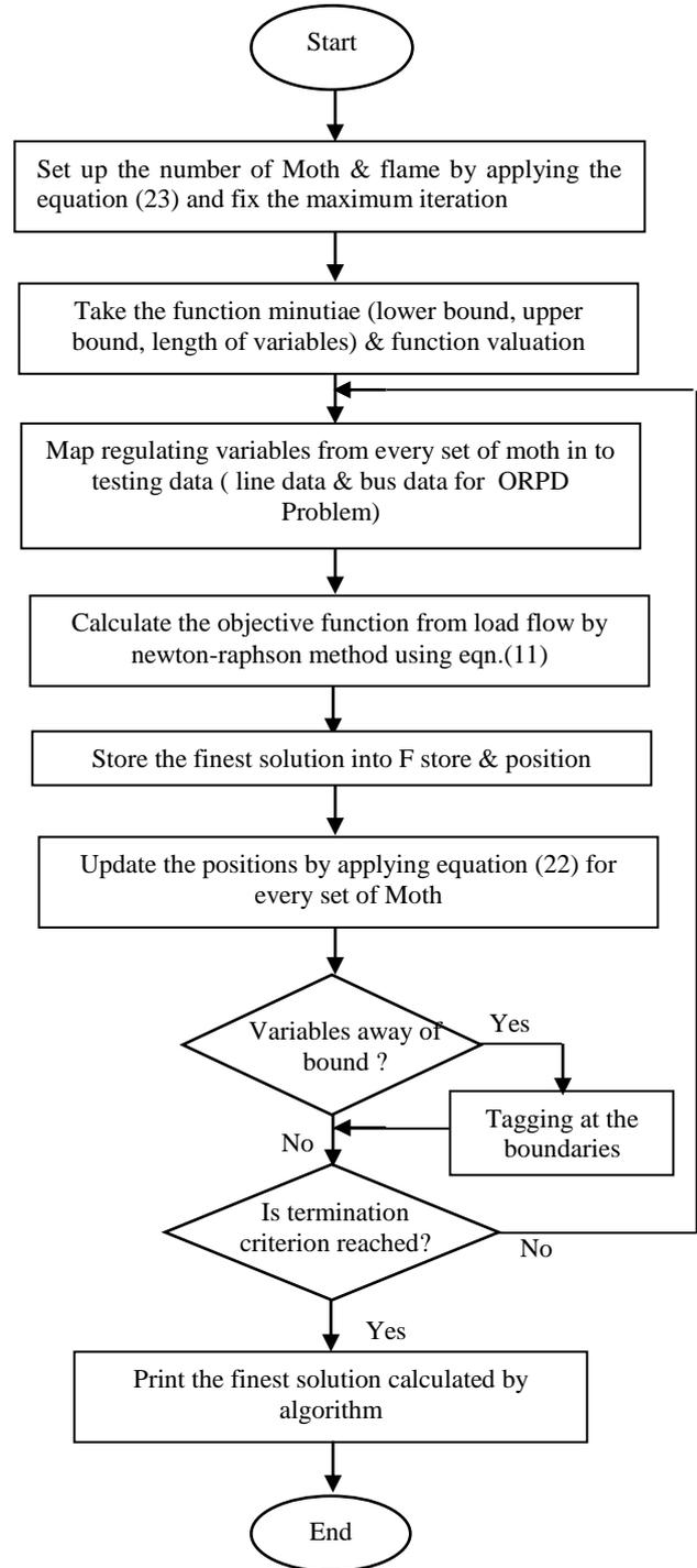
Figure - 6 Flow chart for MFO algorithm
