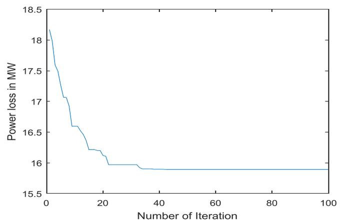
**Figure -7** Convergence characteristics of 30-bus system
