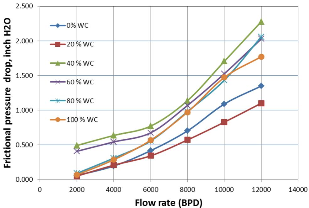
**Figure 3b:** Effect of flow rate on pressure drop for different water cuts ( $0^\circ$  case).
