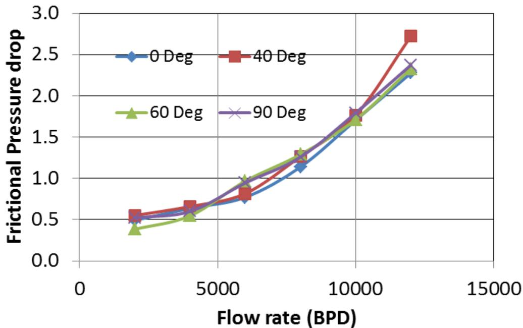
Figure 7a: Effect of inclination on pressure drop for different flow rates (40% WC).
