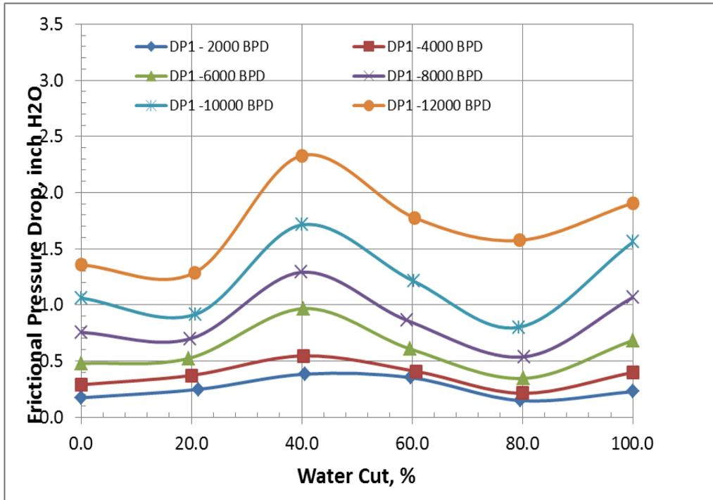
Figure 5a: Effect of water cut on pressure drop for different flow rates (60° case).
