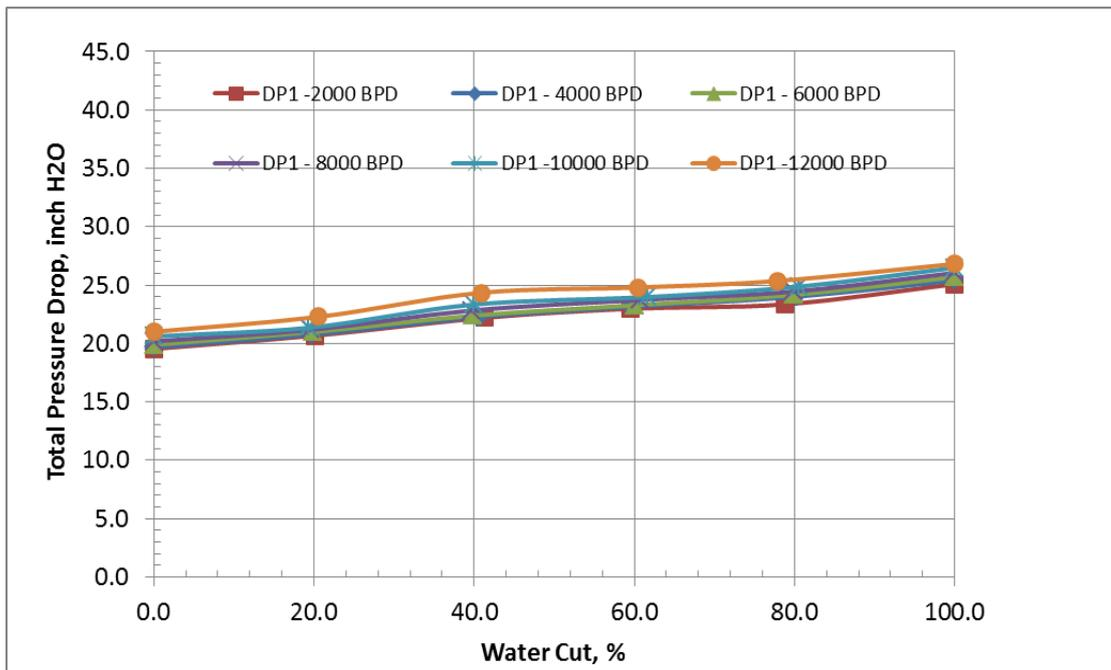
**Figure 8a:** Effect of inclination on total pressure drop for different flow rates and water cuts (40 Deg.).
