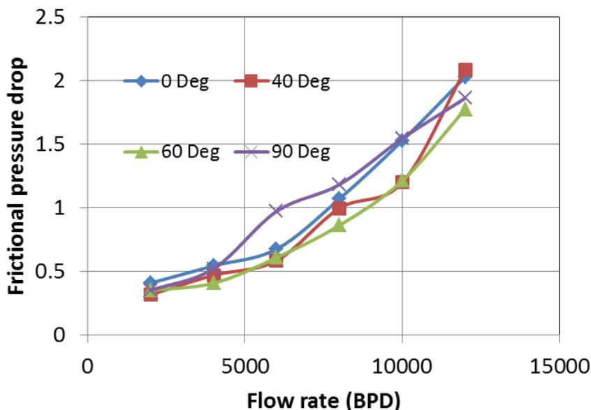
Figure 7b: Effect of inclination on pressure drop for different flow rates (60% WC).
