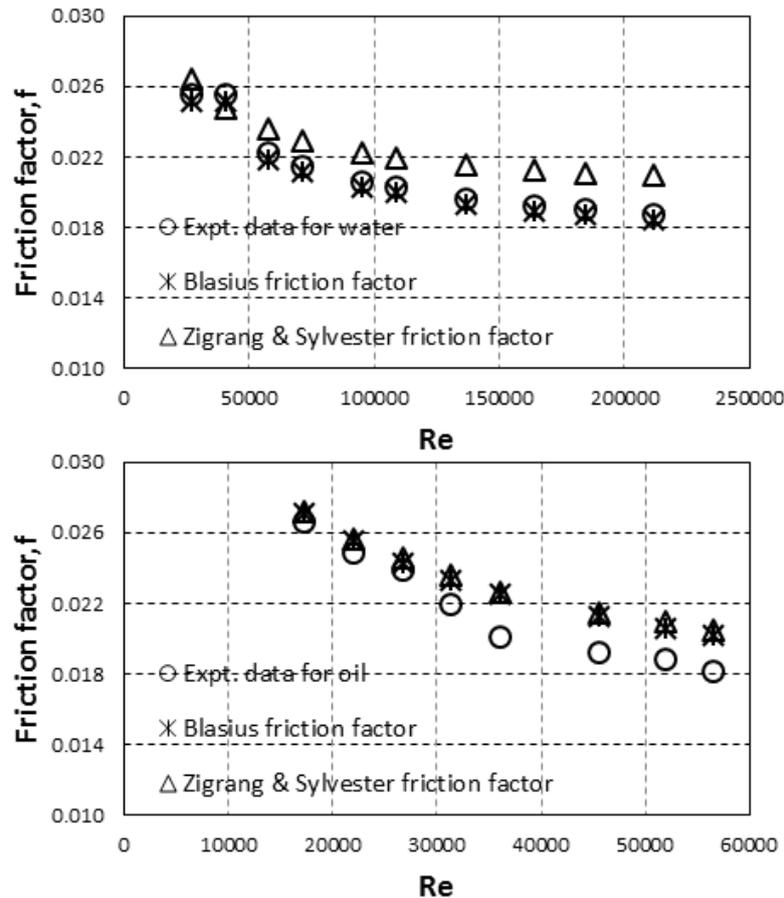
**Figure 2.** Friction factor comparisons with Blasius correlation and Zigrang & Sylvester correlations for oil-water.
