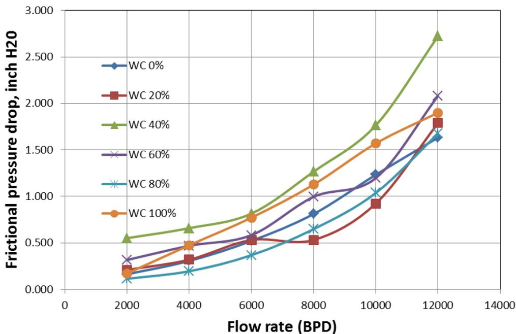
Figure 4b: Effect of flow rate on pressure drop for different flow rates (40° case).
