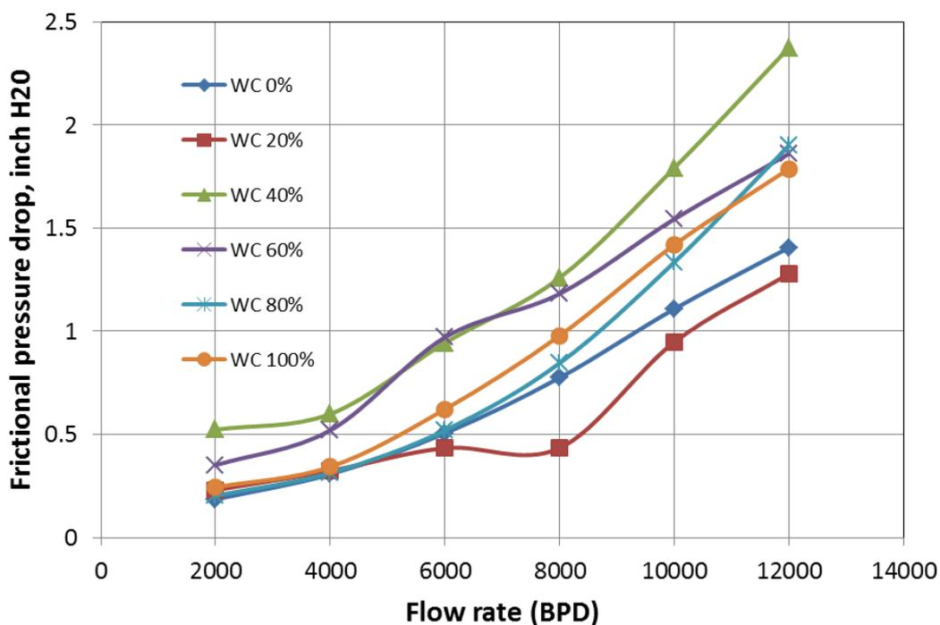
Figure 6b: Effect of flow rate on pressure drop for different flow rates (90° case).
