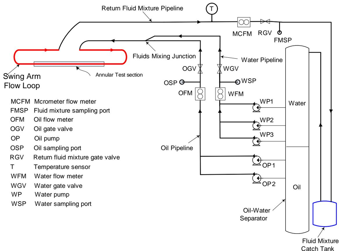
**Figure 1a:** Schematic layout of the oil-water multiphase flow loop.
