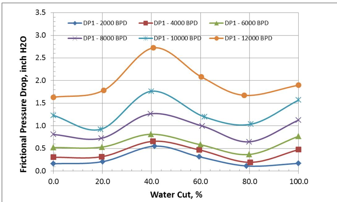
Figure 4a: Effect of water cut on pressure drop for different flow rates (40° case).
