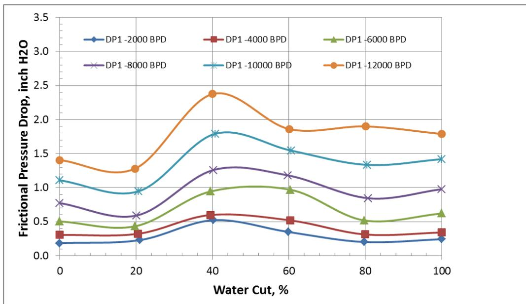
Figure 6a: Effect of water cut on pressure drop for different flow rates (90° case).
