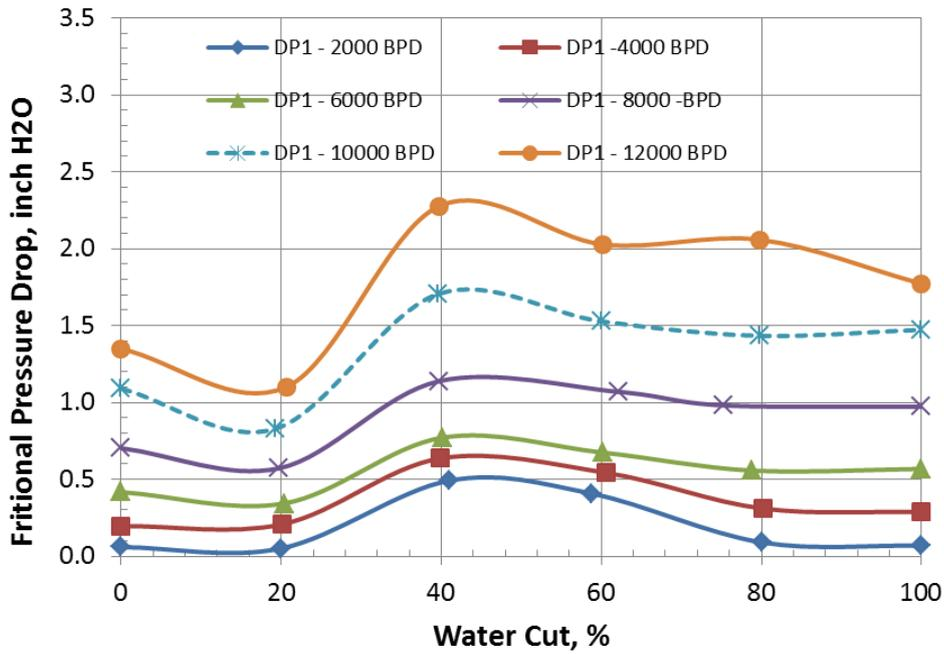
**Figure 3a:** Effect of water cut on pressure drop for different flow rates ( $0^\circ$  case).
