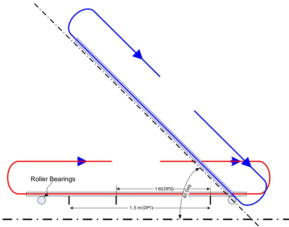
**Figure 1b:** Details of pressure tapping point (DP1 and DP2).
