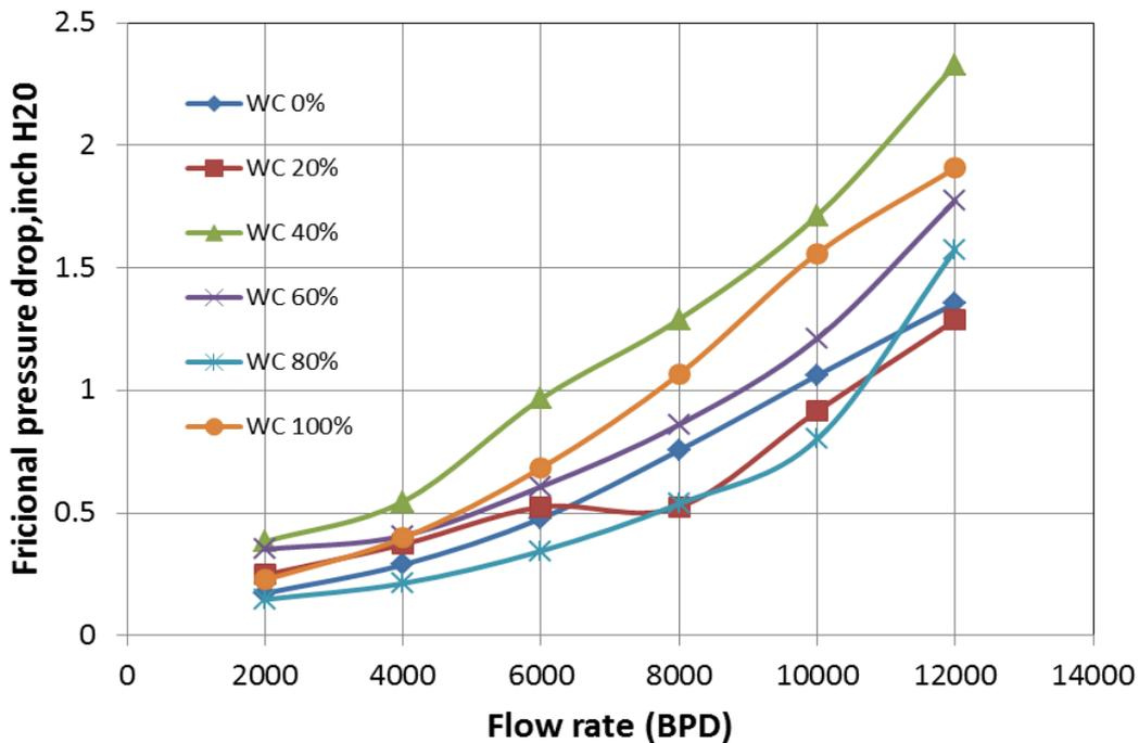
Figure 5b: Effect of flow rate on pressure drop for different flow rates (60° case).
