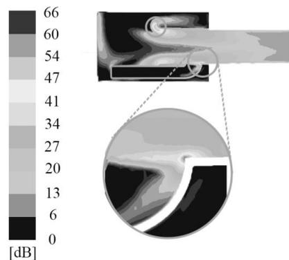
(b) Flow noise in air cleaner XY plane
