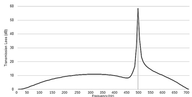
**Figure 5:** Transmission loss of normal air cleaner
