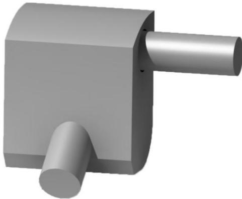
(a) Analysis model of internal flow of air cleaner
