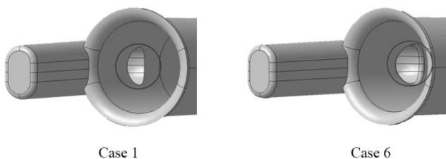
**Figure 5:** Differences in shape of the resonator mount
