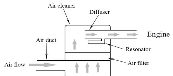
Figure 1: Simple structural diagram of an air cleaner
