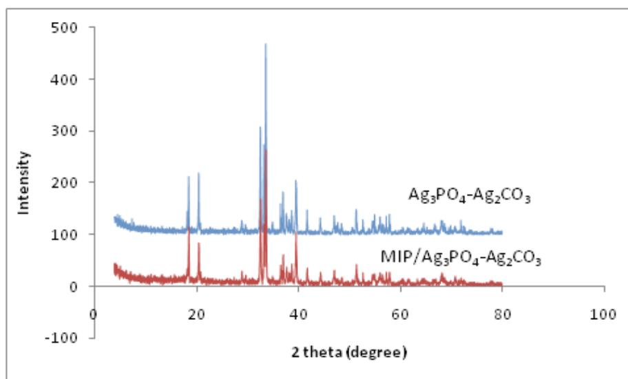
**Figure 1:** XRD patterns of prepared catalyst
