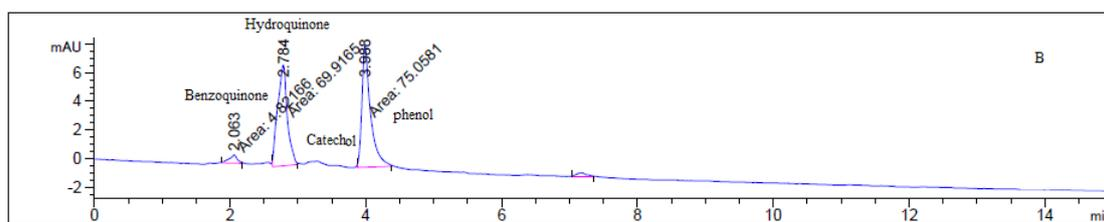
**Figure 6:** HPLC chromatogram of phenol (a) before and (b) after degradation under sunlight.
