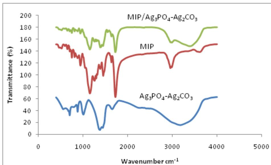
**Figure 2:** FTIR curves of the prepared materials
