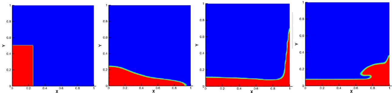
**Figure 5:** Break dam with interfacial sharpening, without mass loss and no interfacial at different time
