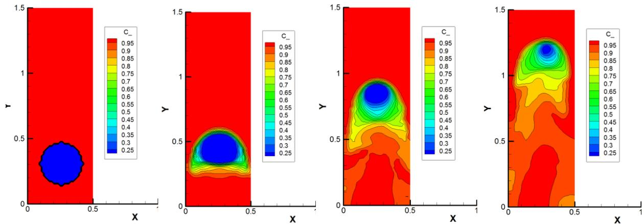
**Figure 3:** Bubble rising without any sharpening, mass loss and interfacial smearing
