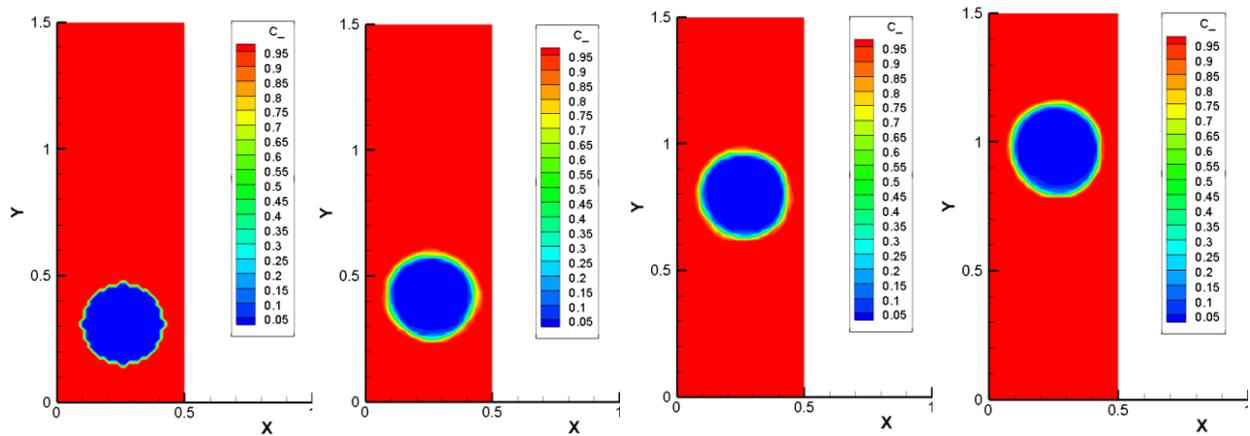
**Figure 4:** Bubble rising with interfacial sharpening, without mass loss and no interfacial smearing
