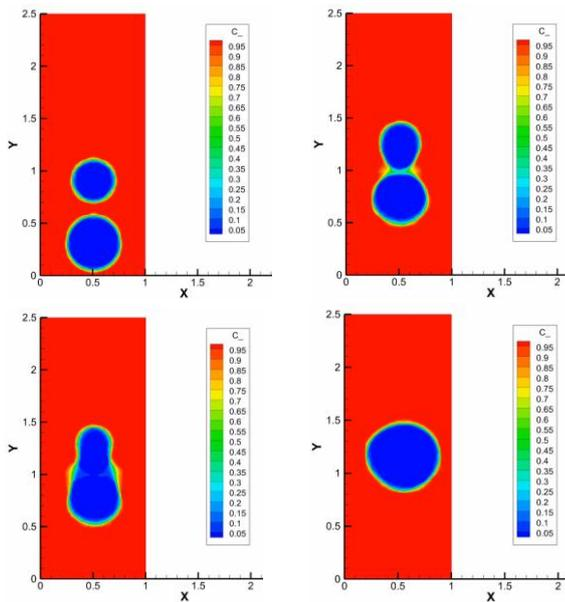
**Figure 6:** Bubbles coalescence with interfacial sharpening.
