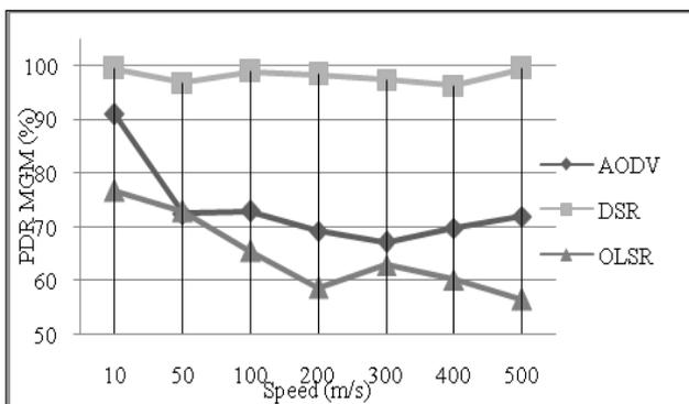
Figure 9. PDR versus speed for MGM.
