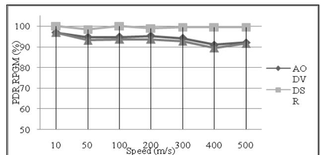
Figure 6. PDR versus speed for RPGM.
