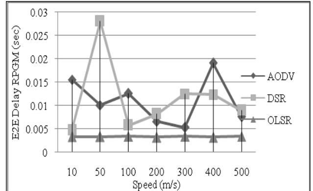
Figure 10. Average E2E delay versus speed for RPGM.
