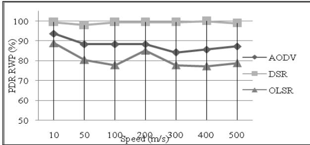
Figure 7. PDR versus speed for RWP.
