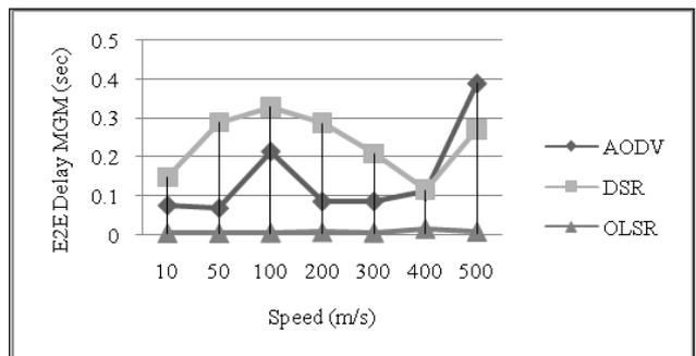
Figure 13. Average E2E delay versus speed for MGM.
