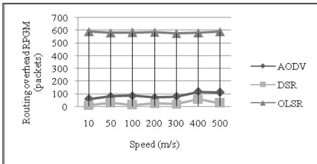
Figure 14. Routing overhead versus speed for RPGM.
