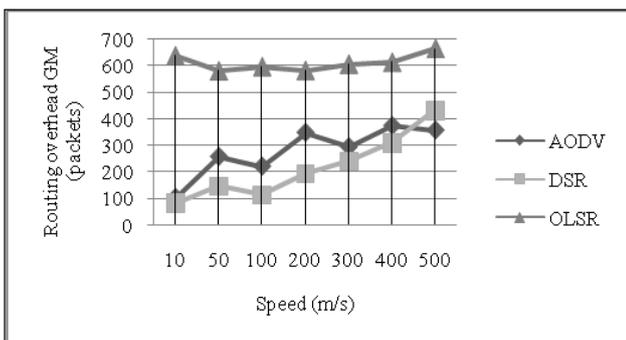
Figure 16. Routing overhead versus speed for GM.
