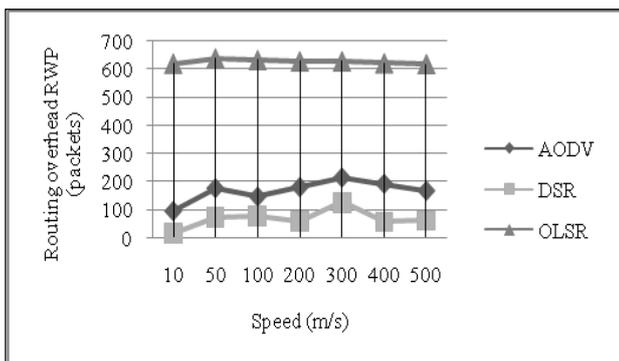
Figure 15. Routing overhead versus speed for RWP.
