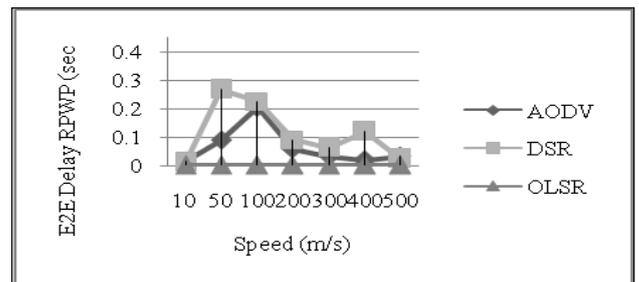
Figure 11. Average E2E delay versus speed for RWP.
