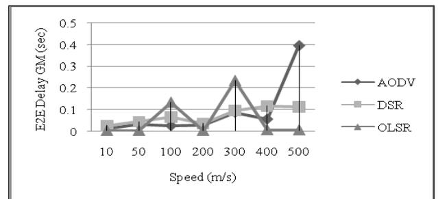
Figure 12. Average E2E delay versus speed for GM.
