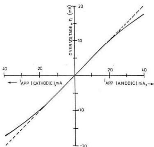
Figure 1: Schematic representation linear polarization curve
