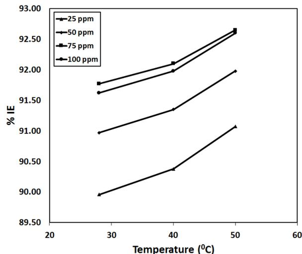
**Figure 7:** Effect of temperatures on %IE of BPTU
