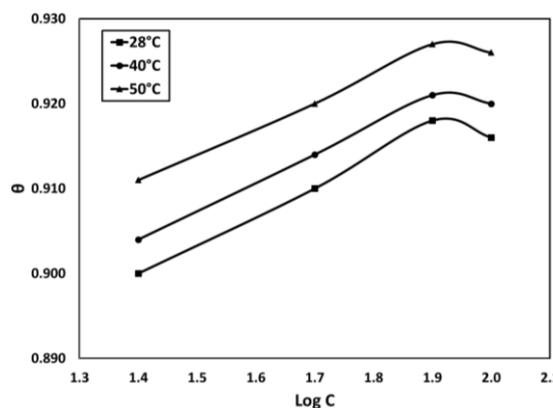
**Figure 8:** Temkin's adsorption isotherm plot for mild steel at different temperatures in 0.1 N H<sub>2</sub>SO<sub>4</sub>
