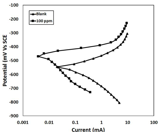
**Figure 5:** Tafel plot of mild steel in 0.1N  $\text{H}_2\text{SO}_4$  with and without BPTU at 28 °C
