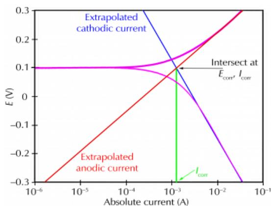
Figure 1: Schematic representation of Tafel plot
