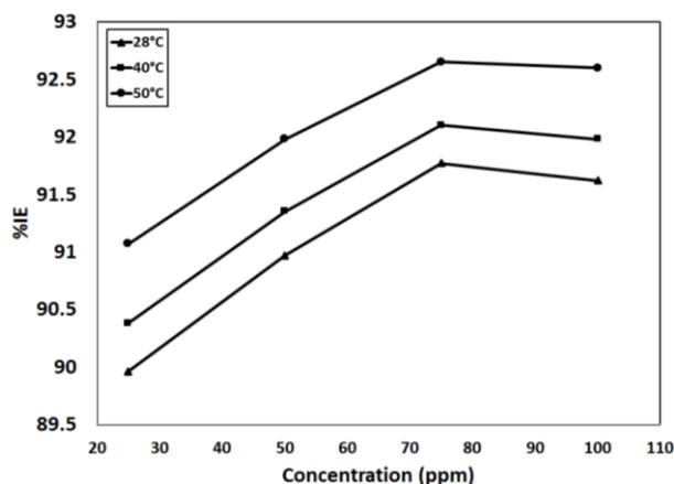
**Figure 6:** Effect of inhibitor concentration on % IE in 0.1 N H<sub>2</sub>SO<sub>4</sub>
