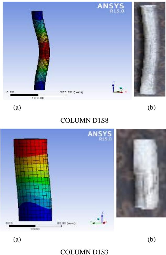
**Figure 6.** Typical (a) FE model and (b) Experimental deformed shapes for columns D1S8 and D1S3
