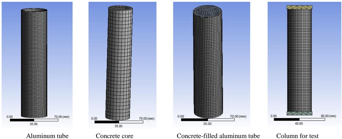
**Figure 1.** Meshing of the concrete-filled aluminum tube columns
