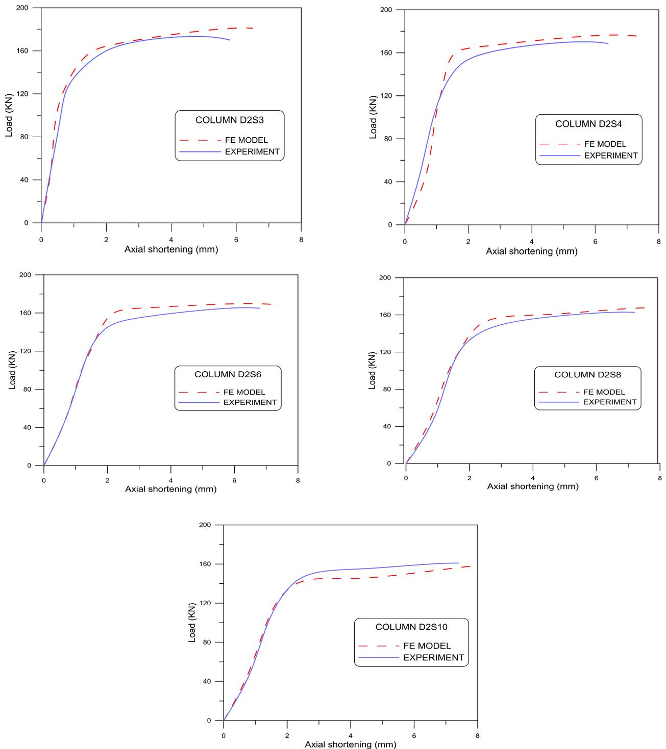
**Figure 5.** Experimental versus current FE model for columns in G1.
