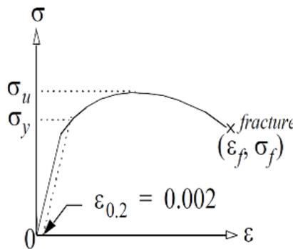
**Figure 4.** Typical stress-strain curve for aluminum tube
