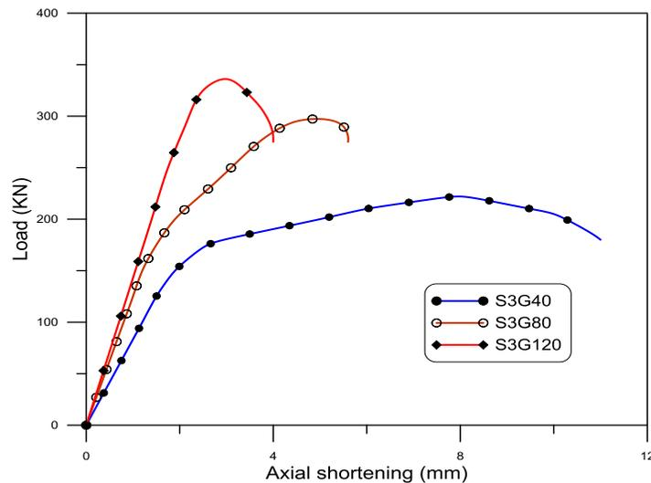
**Figure 7.** Load- Axial shortening curves for high grade concrete infill specimens
