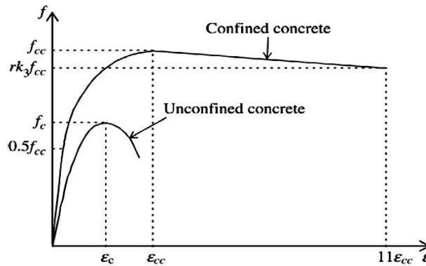
**Figure 3.** Stress-strain curves for both confined and unconfined concrete
