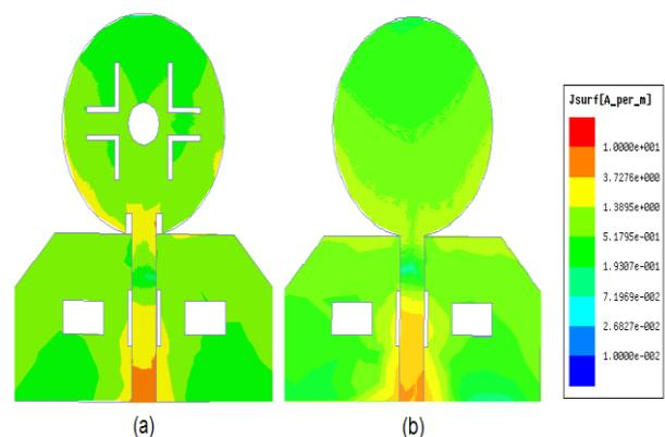
**Figure 3.** Current distribution at 3.3 GHz (a) In proposed Antenna (b) Simple Disc
