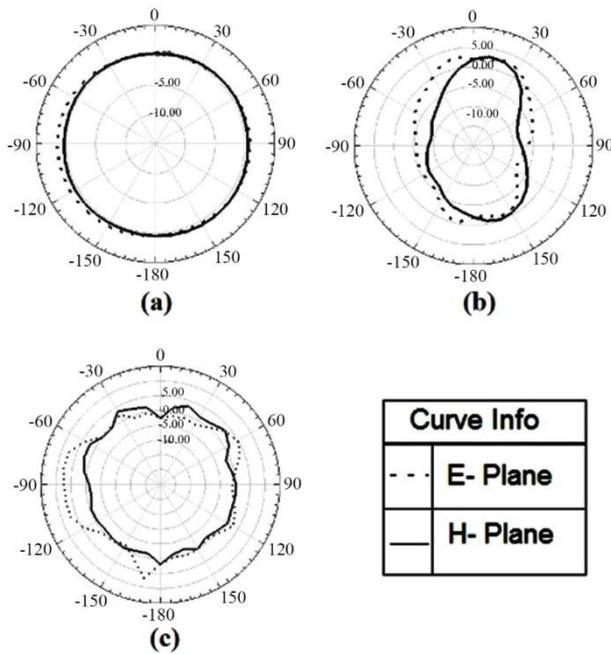
**Figure 6.** Measured Radiation pattern of proposed antenna (a) 3.3 GHz (b) 7.0 GHz (c) 9.2 GHz
