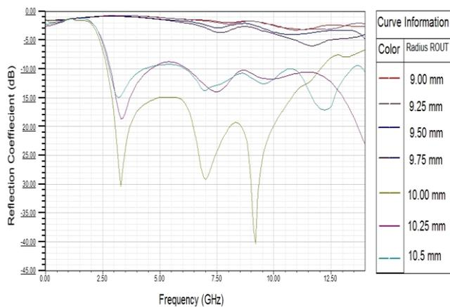
**Figure 4.** Variation in reflection coefficient of proposed antenna with ROUT.
