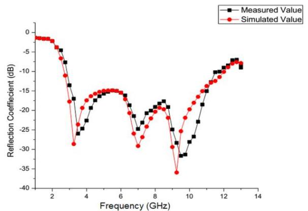
**Figure 2.** Comparison between simulated and measured reflection coefficient
