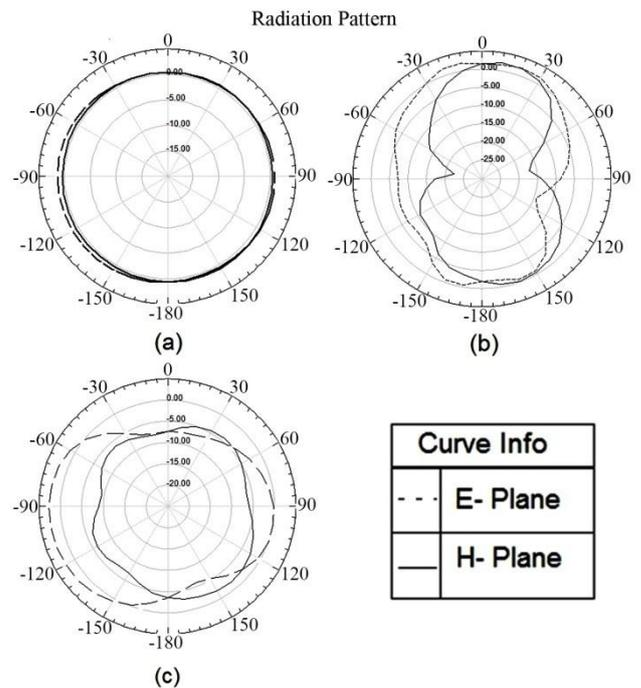
**Figure 5.** Simulated Radiation pattern of proposed antenna (a) 3.3 GHz (b) 7.0 GHz (c) 9.2 GHz
