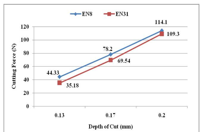
Figure 5. Depth of cut Vs cutting force
