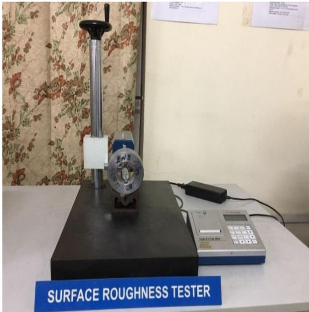
Figure 4. SE-1200 surface roughness tester
