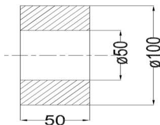
Figure 1. Dimensions and shape of specimen
