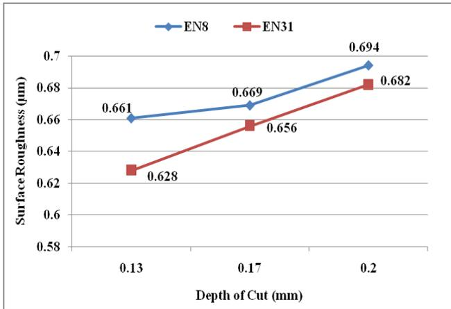
Figure 6. Depth of cut Vs surface roughness
