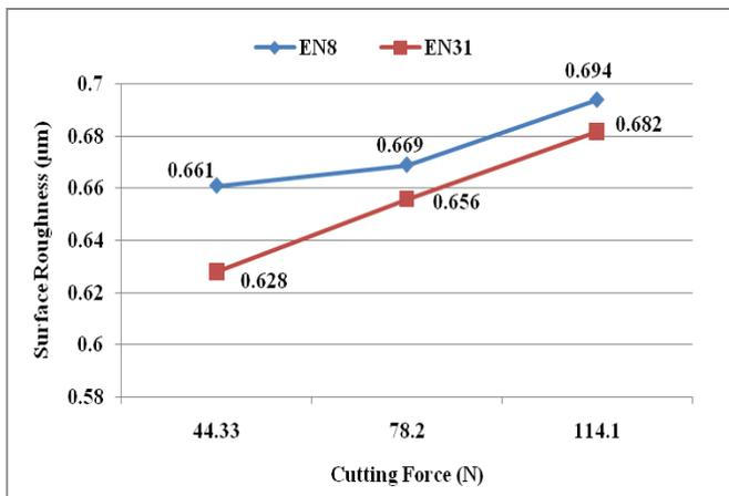
Figure 8. Cutting force Vs surface roughness
