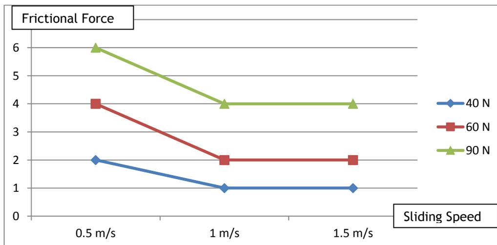
**Figure 3:** Variation in force of friction with the sliding speed
