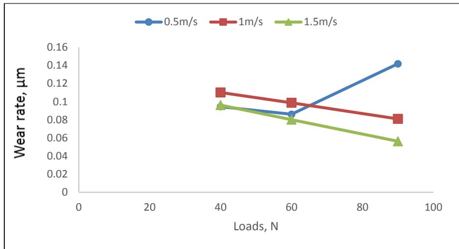
**Figure 10:** Wear rate Vs Load for Wet Test at different sliding speeds
