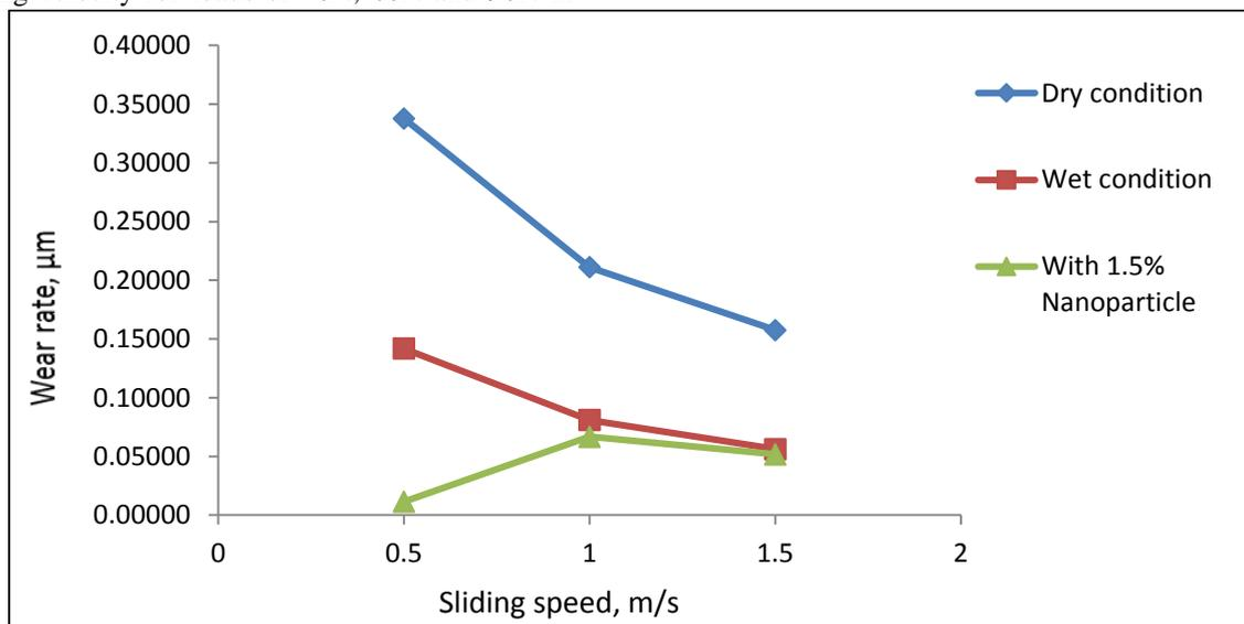
**Figure 11:** Wear rate versus sliding speed in no lubricant, with lubricant and with nanolubricant
