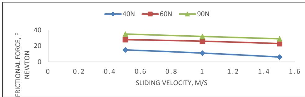
**Figure 1:** Frictional force Vs sliding speed in dry condition at loads 40N, 60 N & 90 N
