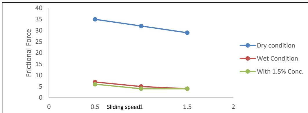
**Figure 8** Force of friction Vs sliding speed in dry, wet and with nanolubricant at load 90 N
