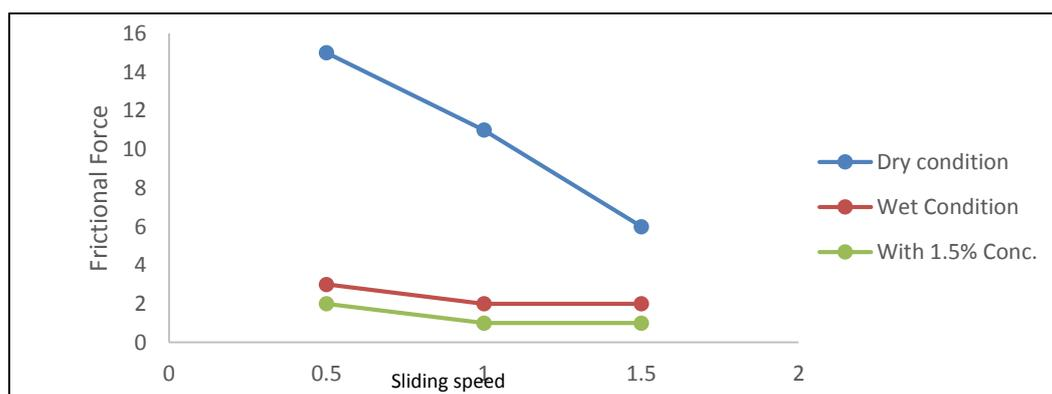
**Figure 6:** Force of friction Vs sliding speed in dry, wet and with nanolubricant at load 40 N
