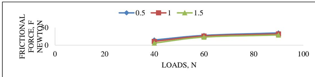
**Figure 4:** Frictional force Vs Load for Dry Condition for different sliding speeds
