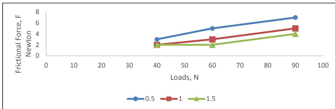
**Figure 5:** Frictional force Vs Load with lubrication oil for different sliding speeds
