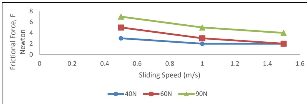
**Figure 2:** Frictional force Vs sliding speed for lubricating oil without nanoadditives
