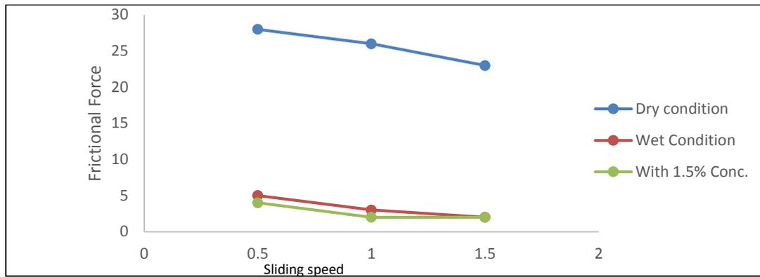
**Figure 7:** Force of friction Vs sliding speed in dry, wet and with nanolubricant at load 60 N
