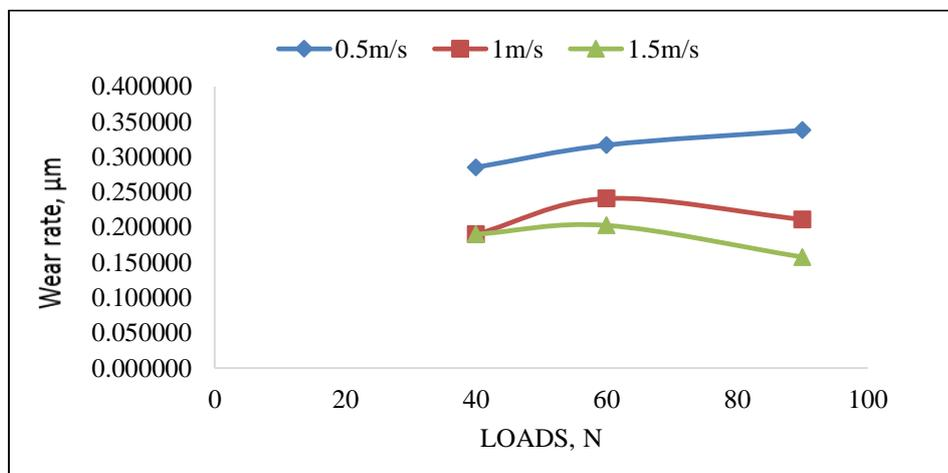
**Figure 9:** Wear rate Vs Load for Dry Test at different sliding speeds
