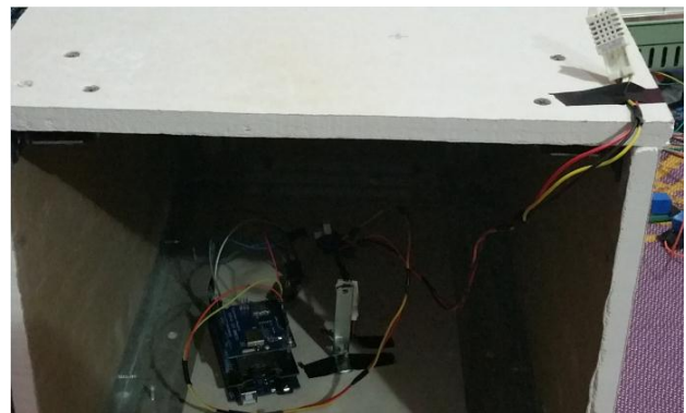
Figure 8 Temperature and humidity sensors inside and outside of the prototype.
