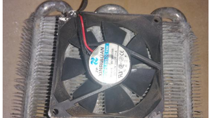
Figure 6. The heat exchanger with fan.
