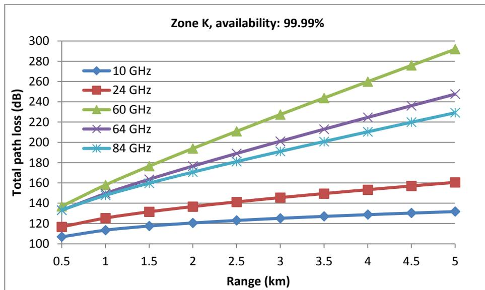
**Figure 4:** Total Path Loss (LOS) Comparison versus Range (km) at Various Frequencies for Rain Zone K (New York) at 4-nine Link Availability (vertical polarization)
