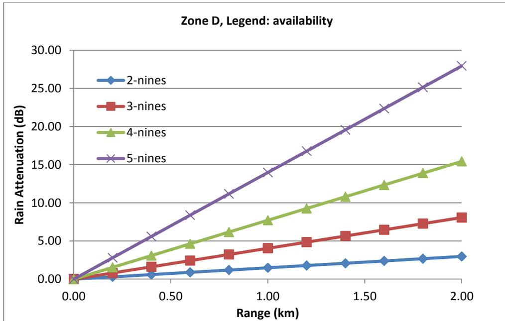
Figure 1: Rain Attenuation vs. Range (km) for Different Link Availability for Region D
