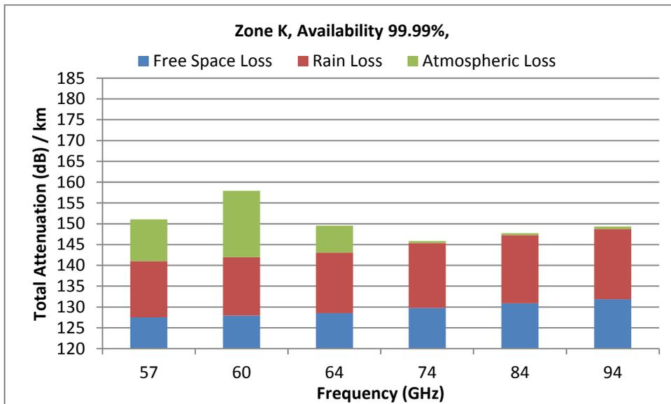
**Figure 9:** Total attenuation (dB) / km breakdown at various frequencies V-band and E-band frequencies for rain Zone K with 99.99% link availability
