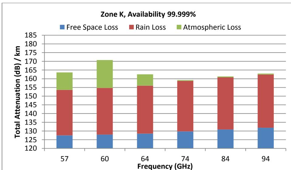
**Figure 10:** Total attenuation (dB) / km breakdown at various frequencies V-band and E-band frequencies for rain Zone K with 99.999% link availability
