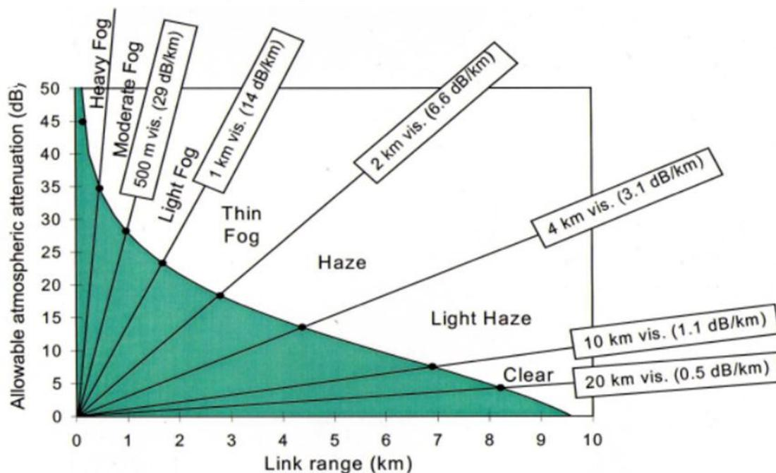
**Figure 8:** An example of allowable FSL link margin curve for atmospheric impairments, intercepted with atmospheric attenuation under different weather conditions [11].
