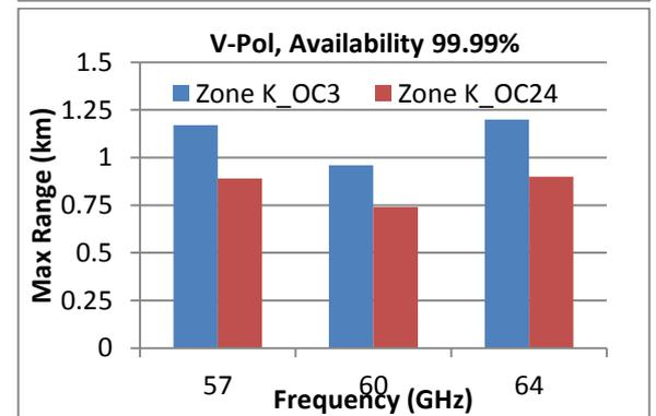
**Figure 6:** Maximum Range Performance versus frequency for rain zone K and data rates OC3 and OC24 (left) 4-nine availability, (right) 5-nine availability
