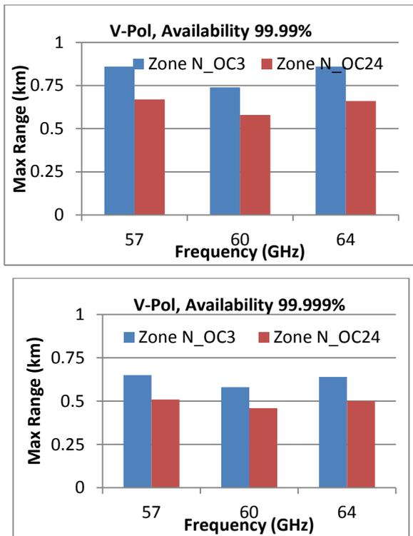
**Figure 7:** Maximum Range Performance versus frequency for rain zone N and data rates OC3 and OC24 (left) 4-nine availability, (right) 5-nine availability
