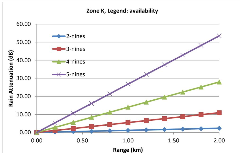
Figure 2: Rain Attenuation vs. Range (km) for Different Link Availability for Region K
