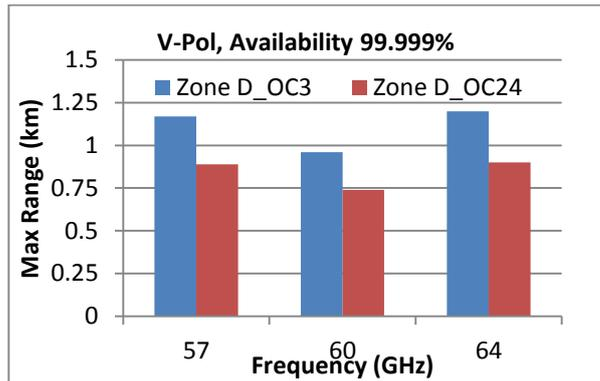
**Figure 5:** Maximum Range Performance versus frequency for rain zone D and data rates OC3 and OC24 (left) 4-nine availability, (right) 5-nine availability
