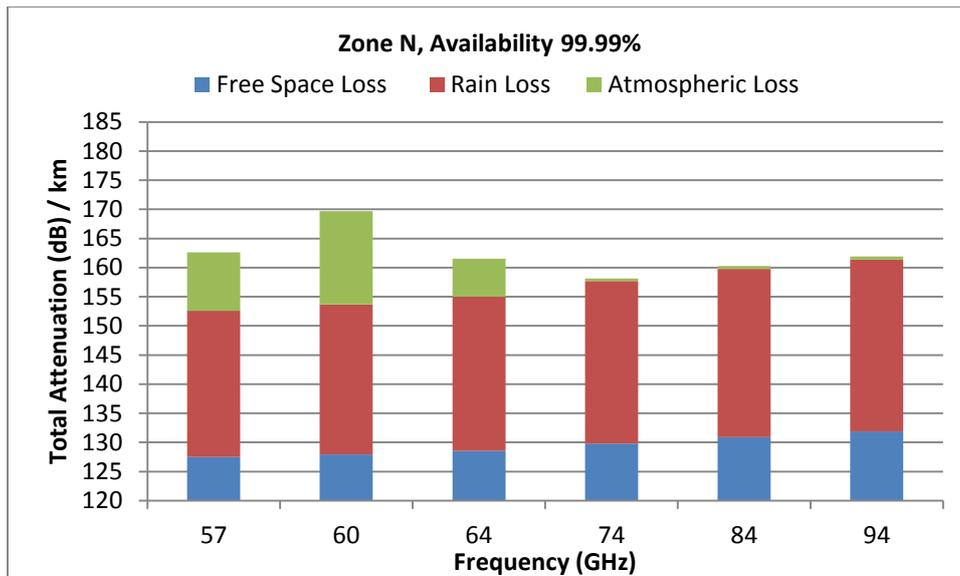
**Figure 11:** Total attenuation (dB) / km breakdown at various frequencies V-band and E-band frequencies for rain Zone N with 99.99% link availability
