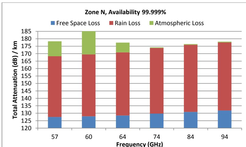
**Figure 12:** Total attenuation (dB) / km breakdown at various frequencies V-band and E-band frequencies for rain Zone N with 99.999% link availability
