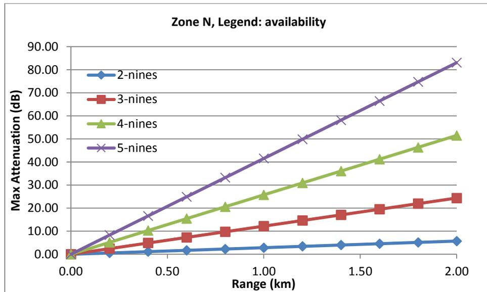
**Figure 3:** Rain Attenuation vs. Range (km) for Different Link Availability for Region N
