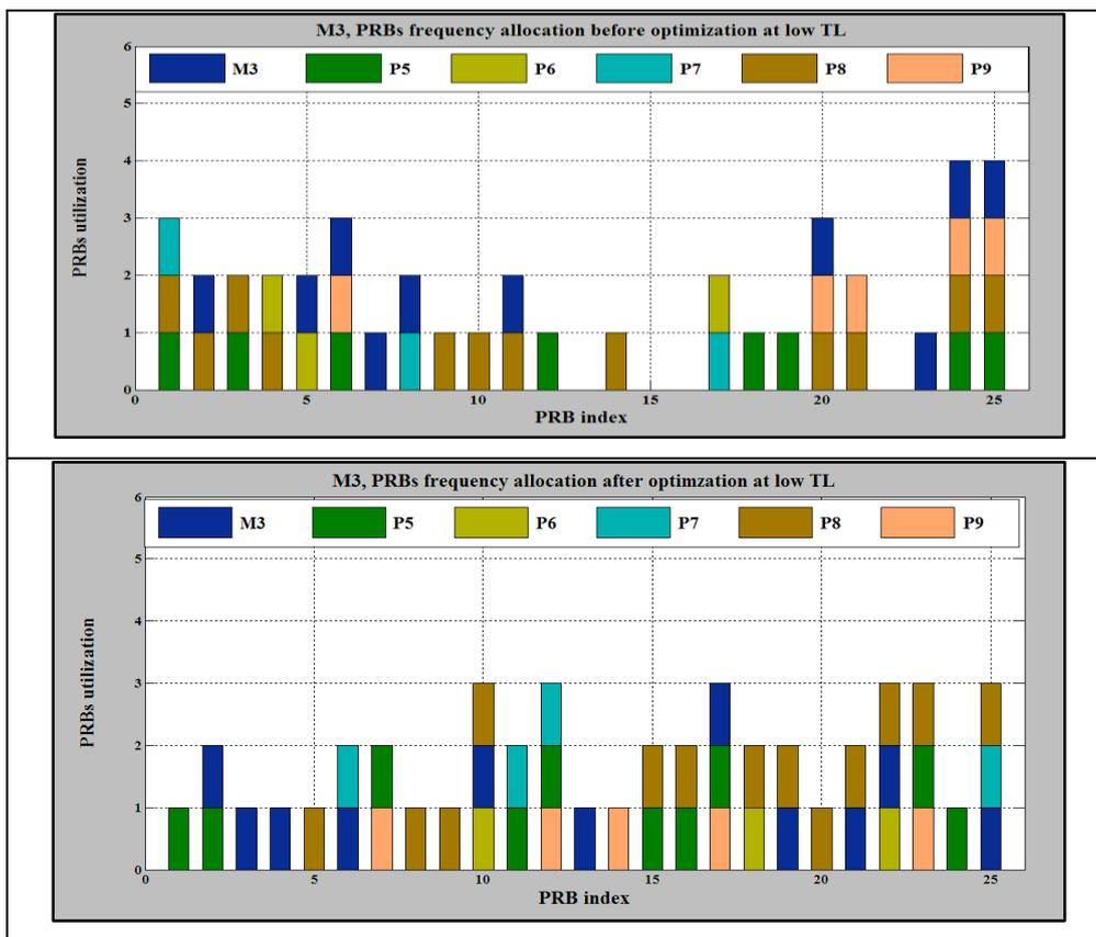
**Figure 4:** PRBs utilization by different M3 HetNet cells at low TL
