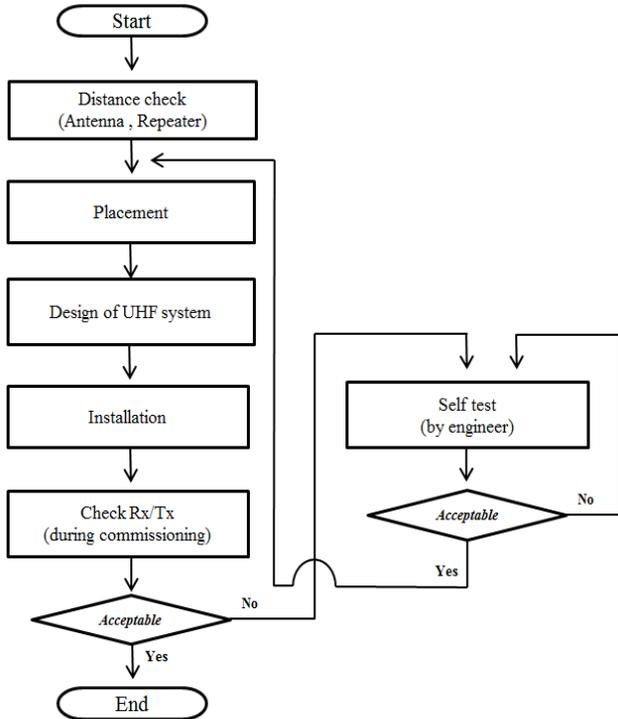
Figure 2: A workflow for the existing UHF system
