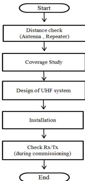
Figure 3: A workflow for the proposed UHF system
