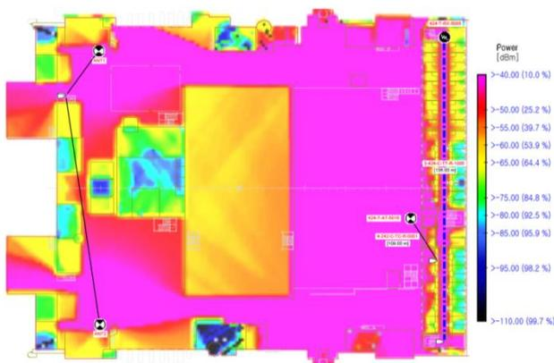
**Figure 10:** The final coverage study at top side
