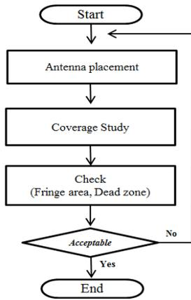
**Figure 5:** A workflow for coverage study of proposed UHF system
