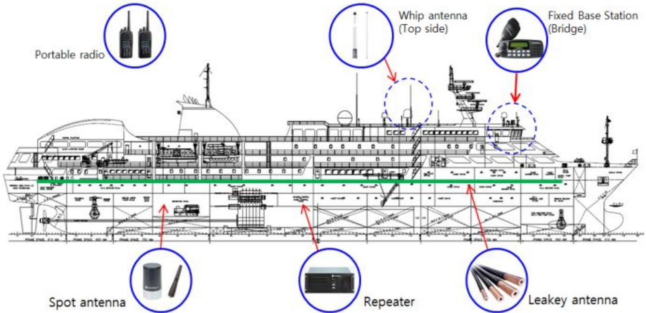
**Figure 1:** Installation of UHF system in ships
