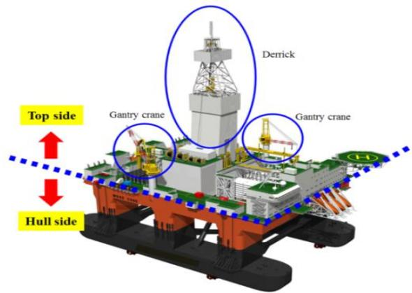
Figure 4: A sample of ship structure
