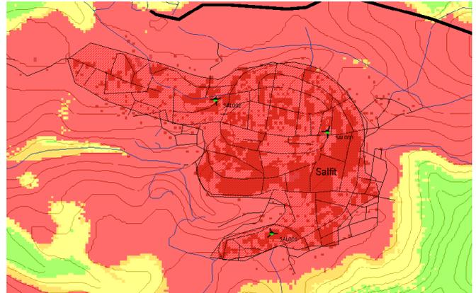
**Figure 2:** Coverage prediction of cellular mobile system.
