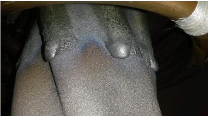
**Figure 2:** The laboratory rotor sample after melting by high-frequency currents
