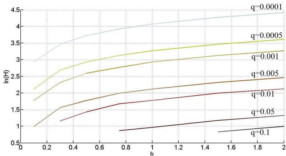
**Figure 6.** The nomogram for determining the optimum depth of the computational domain H for the case  $h \in [0.1; 2]$ ,  $l = 3$
