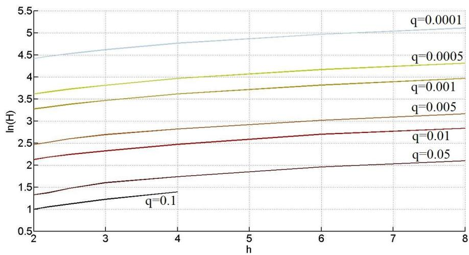
**Figure 5.** The nomogram for determining the optimum depth of the computational domain H for the case  $h \in [2; 8]$ ,  $l = 3$
