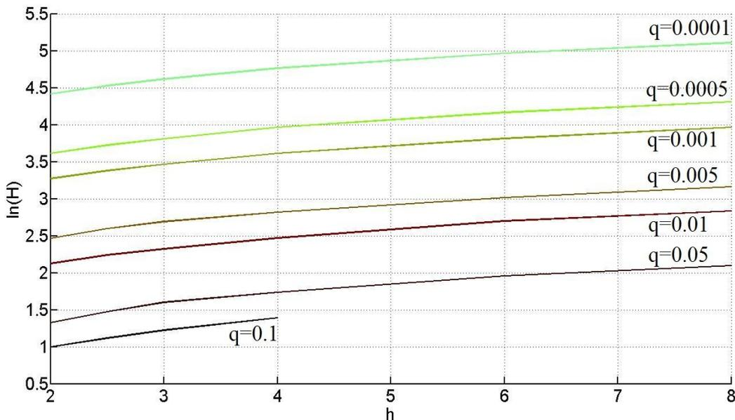
**Figure 3.** The nomogram for determining the optimum depth of the computational domain H for the case  $h \in [2; 8], l = 1$
