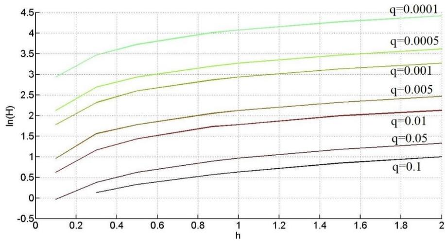
**Figure 4.** The nomogram for determining the optimum depth of the computational domain H for the case  $h \in [0.1; 2]$ ,  $l = 1$
