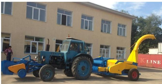
**Figure 5** - General view of the experimental model of detachable pickup with universal pickup-chopper with width of 1.8 m (side view)
