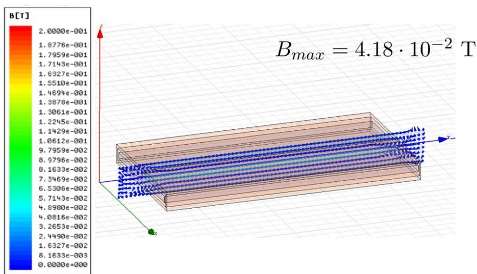
**Figure 7.** Magnetic field density inside the material.
