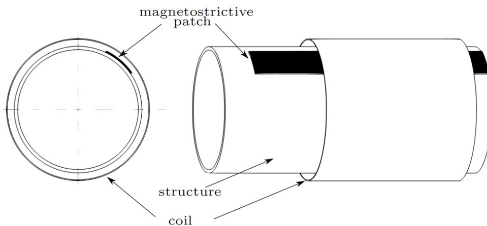
**Figure 2.** A solution of traditional magnetostrictive patch devices [17].
