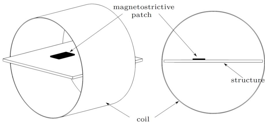
**Figure 3.** A solution of traditional magnetostrictive patch devices [18].
