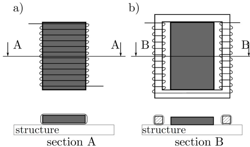
**Figure 4.** Layouts of traditional configuration (a) and innovative solution (b).
