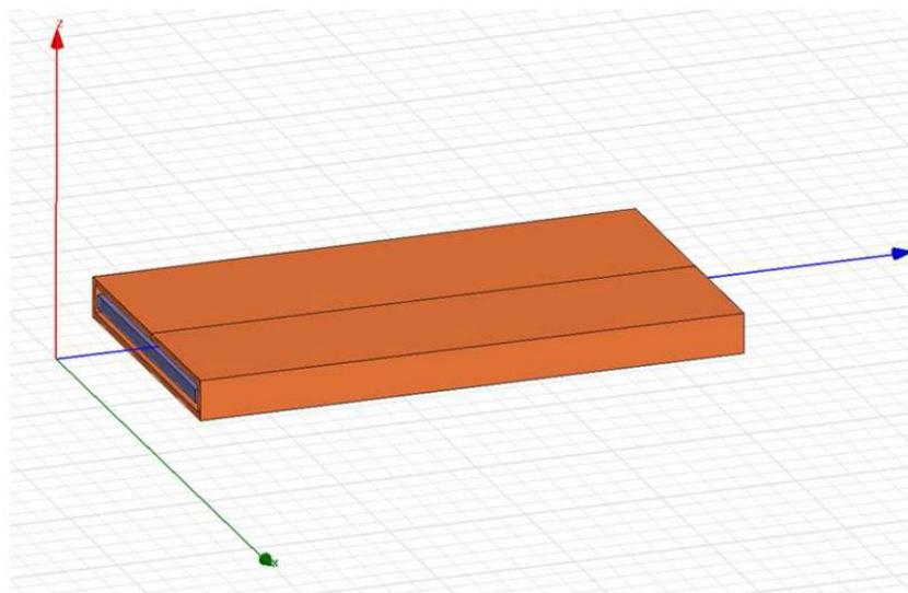
**Figure 6.** Magnetostrictive patch actuator: traditional layout.
