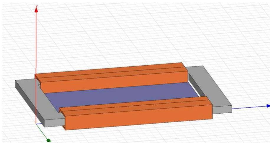
**Figure 8.** Magnetostrictive patch actuator: innovative layout.
