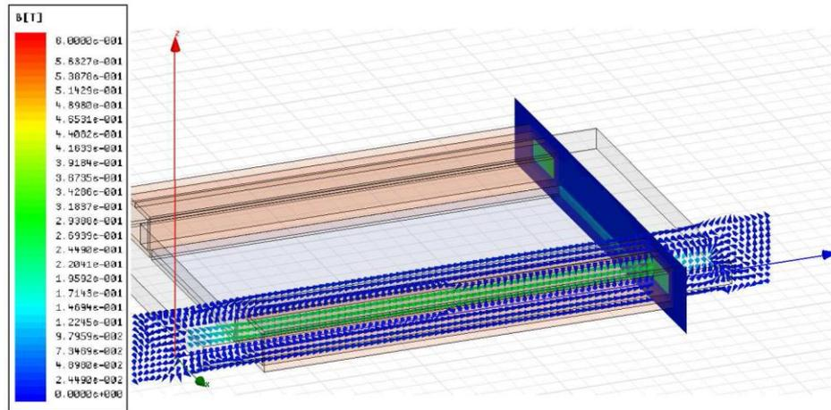
Figure 10. Magnetic field density inside the material: cross section.
