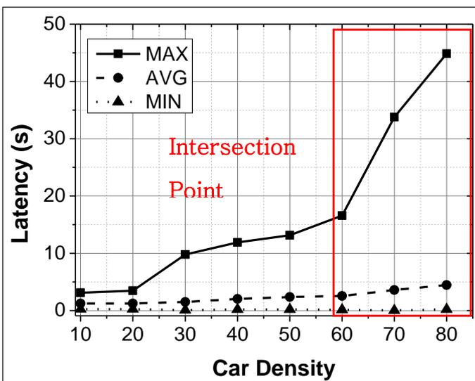
**Figure 5:** Maximum, Average, Minimum Latency each Car Density at Duty Cycle 10%
