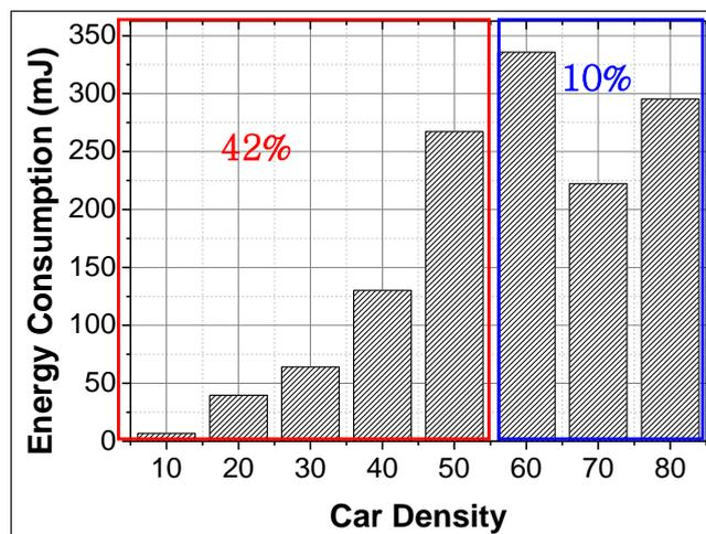
Figure 8: Energy Consumption each Car Density at Fusion of Duty Cycle 10% and 42%
