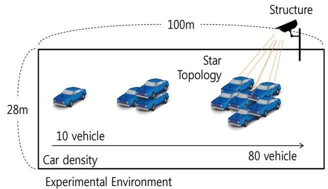
**Figure 2:** Experimental Environment in Smart Traffic
