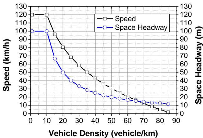
**Figure 1:** Relationship of speed, space headway, and vehicle density
