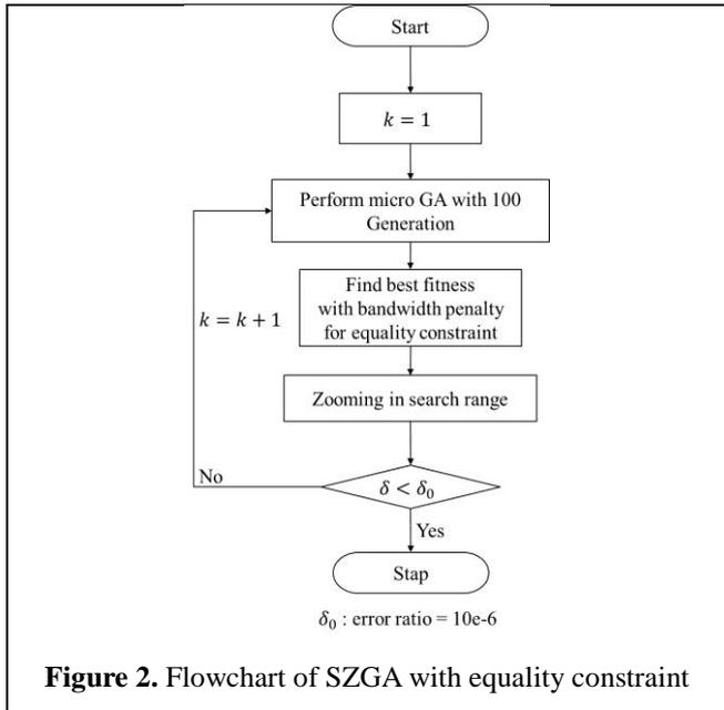
**Figure 2.** Flowchart of SZGA with equality constraint
