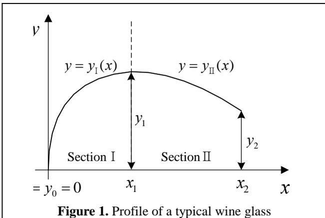
Figure 1. Profile of a typical wine glass
