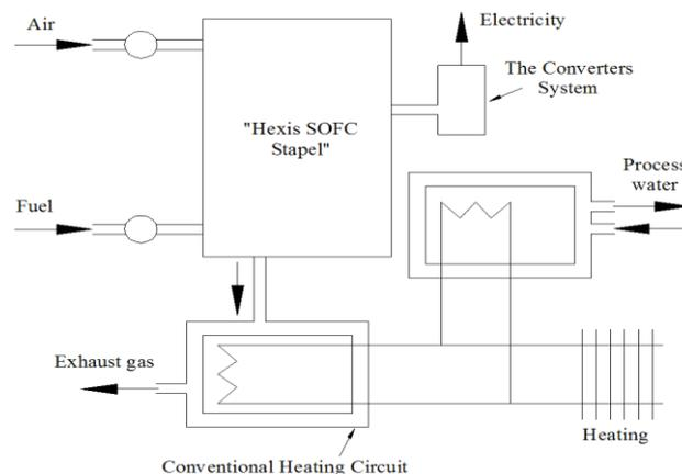
**Figure 1:** Schematic diagram of «Hesis» SOFC-based mini-CHP
