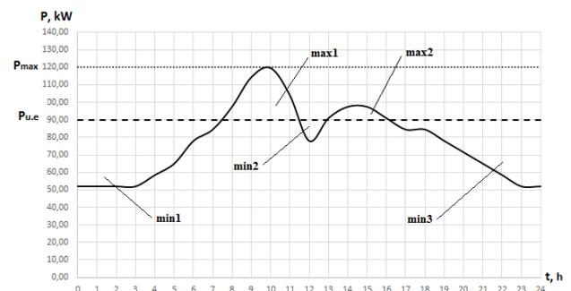
**Figure 2:** The agricultural enterprises daily load schedule of SOFC-based mini-CHPs power supply system
