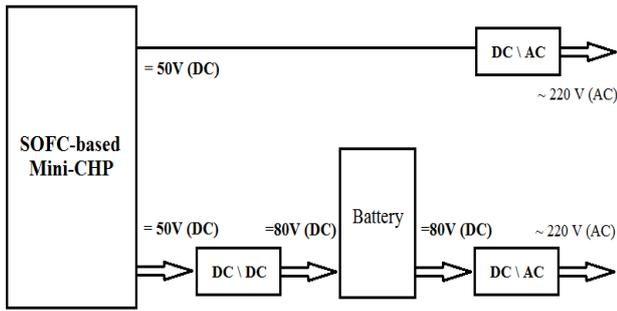
Figure 3: Block diagram of conversion subsystem
