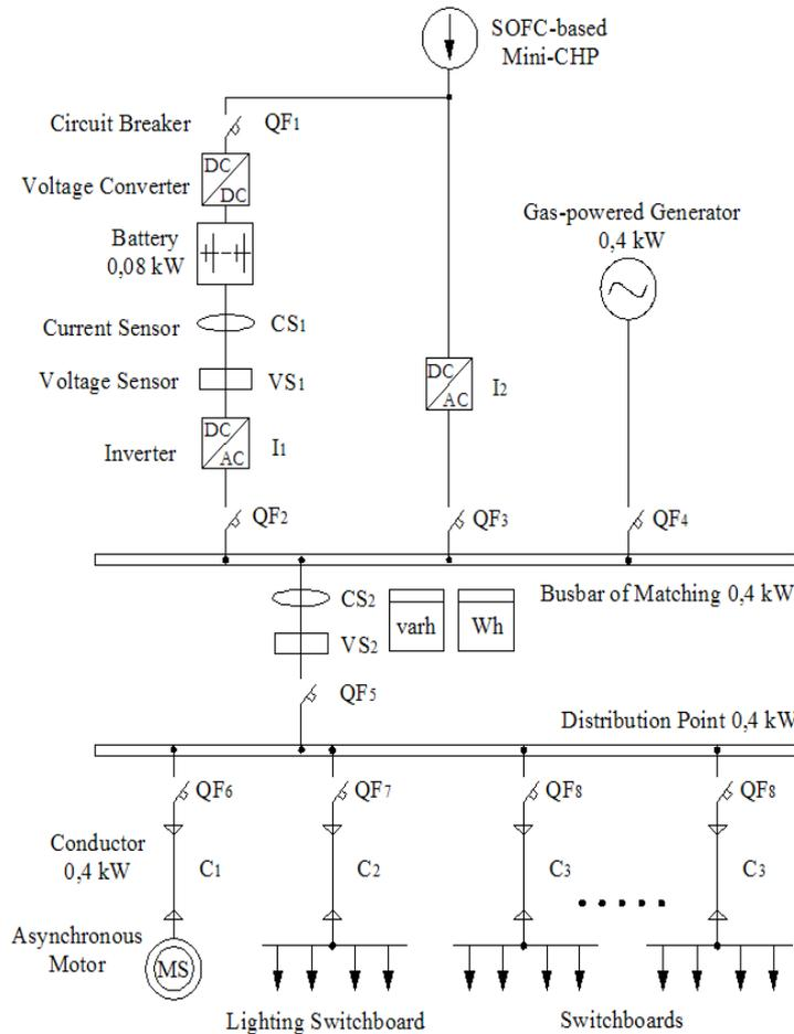
Figure 4: Single-line diagram of SOFC-based mini-CHP power supply system of remote agricultural enterprise
