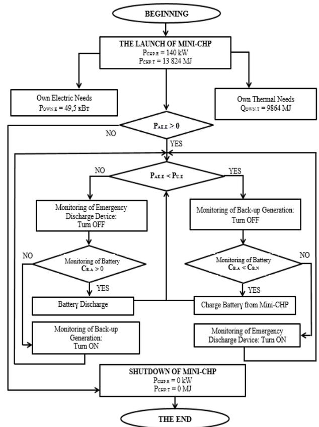
Figure 5: The block diagram of the algorithm
