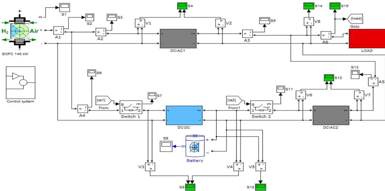
Figure 6: Primary Simulink model for agricultural enterprises power supply system based mini-CHP
