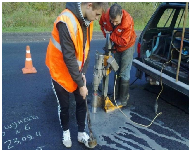
Figure 4. Sampling of asphalt concrete pavement on pilot site
