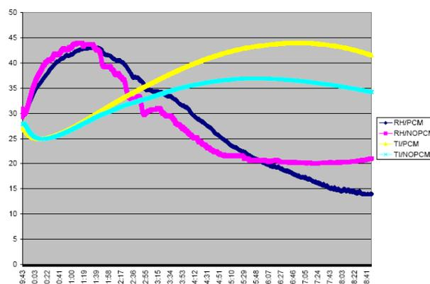
**Figure 6.** Comparison of inside air temperature and the relative humidity for the two designed rooms, 04.03.2016.
