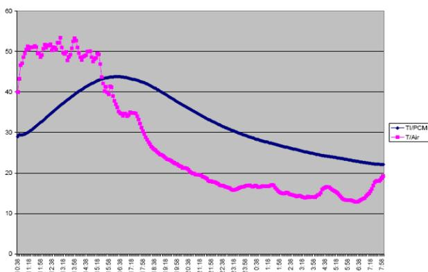
**Figure 4.** Comparison of inside and outside air temperature for the designed room with PCM, 02.03.2016..
