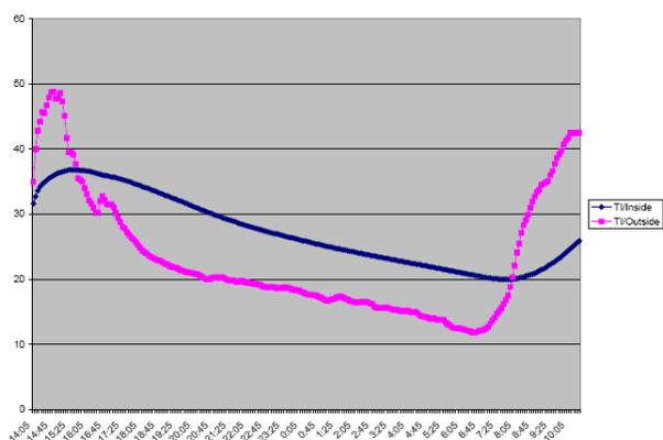
**Figure 5.** Comparison of inside and outside air temperature for the designed room with PCM, 03.03.2016.
