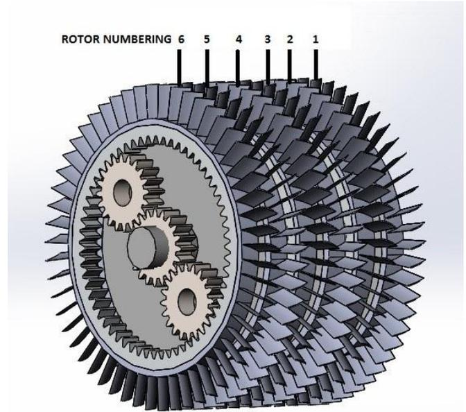
Figure 4: Single shaft contra rotating axial compressor
