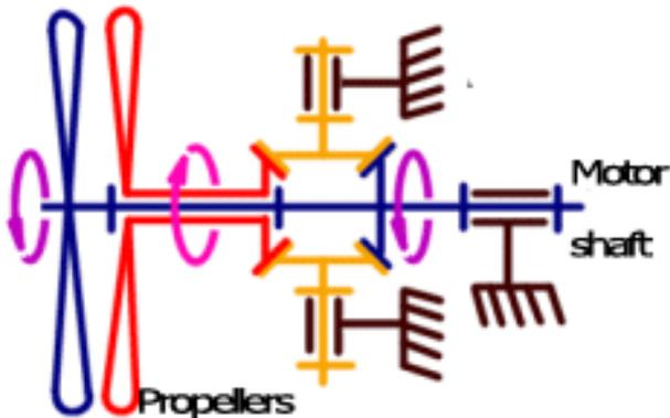
Figure 3: “Coaxial Contra rotating propeller”
