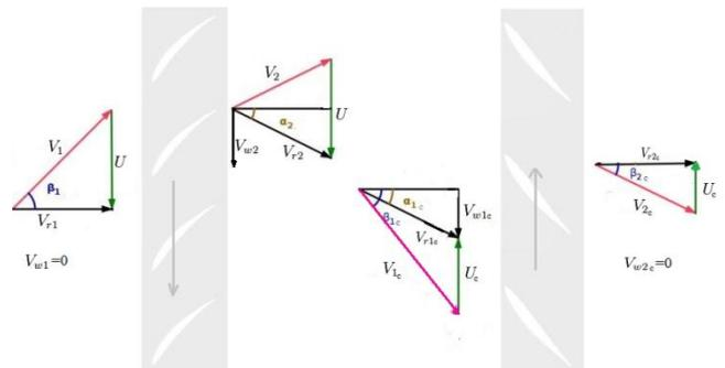
Figure 8: Velocity triangles of single shaft contra rotating compressor.
