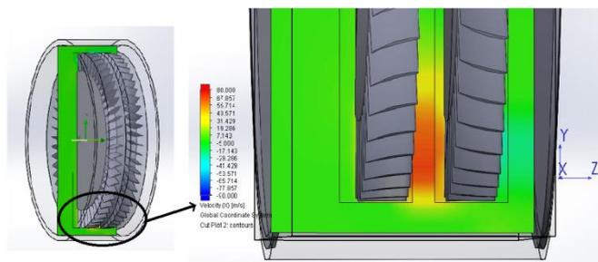
Figure 7: Variation of tangential velocity across single stage contra rotating compressor blades
