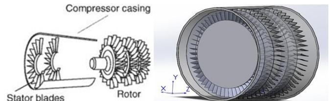
**Figure 1:** Traditional Axial Compressor
