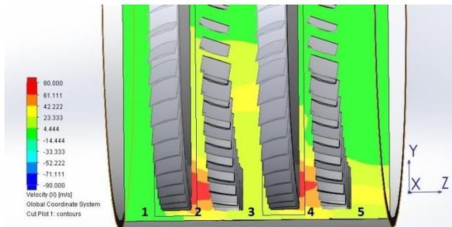
**Figure 9:** Variation of tangential velocity across two stage traditional compressor
