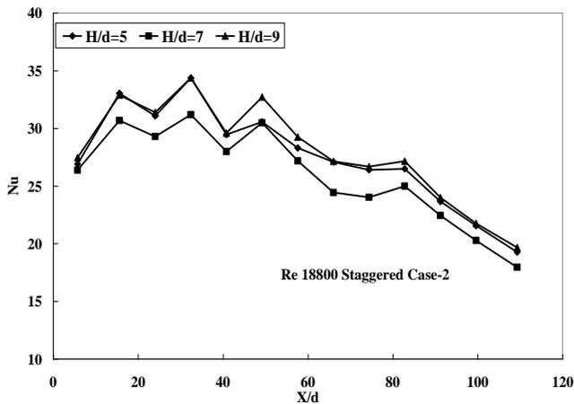
**Figure 7:** Nusselt number distribution for different aspect ratios and for outflow orientation opposing the entry flow (for jet-orifice plate with staggered holes and for Re =18800)
