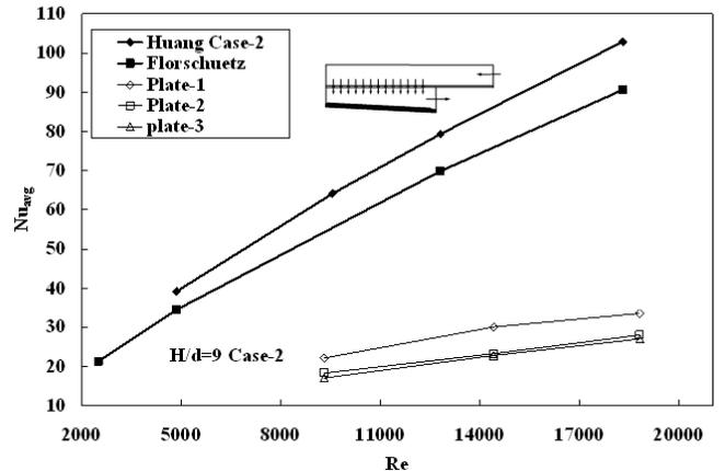
**Figure 10:** Comparison of Average Nusselt number of present study with archival studies for different jet Re and for different orifice-jet configurations (for H/d=9, for outflow opposing entry flow)
