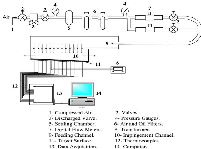
Figure 1: Schematic of the test section
