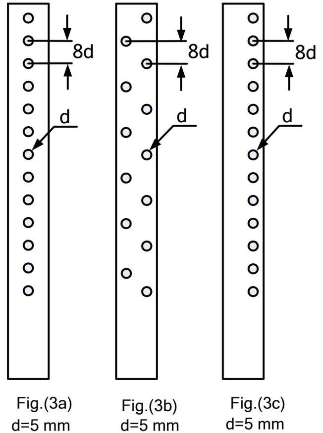
Figure 3: Illustration of three orifice-jet configurations with single array of jets ( $d = 5 \text{ mm}$ ) (Fig. 3a Centered holes, Fig. 3b Staggered holes, Fig. 3c Tangential holes)
