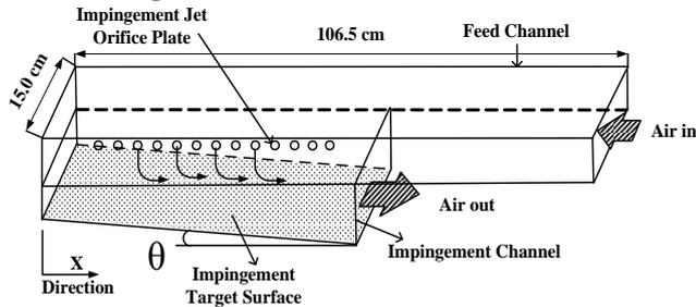
Figure 2.1: Three-dimensional view of the test section
