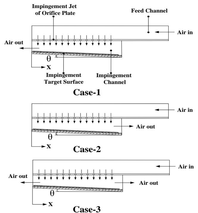
**Figure 4:** Illustration of three exit outflow orientations
