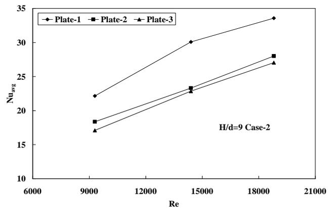
**Figure 9:** Average Nusselt number distribution for different jet Re and for different orifice jet-plate configurations (for aspect ratio H/d=9, for outflow orientation opposing the entry flow)
