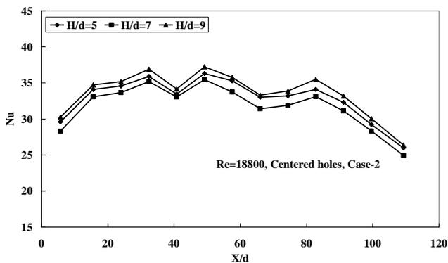
**Figure 6:** Nusselt number distribution for different aspect ratios and for outflow orientation opposing the entry flow (for jet-orifice plate with centered holes and for Re =18800)
