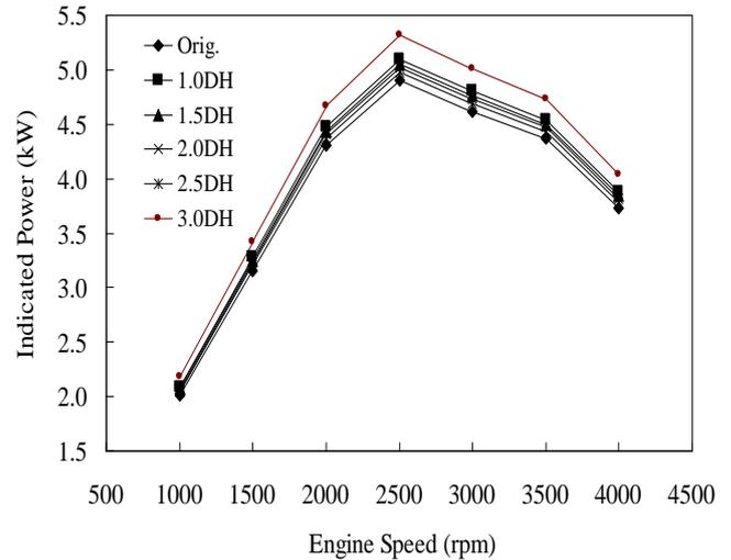
(a). Indicated power of new multi-diameter hole injector nozzles
