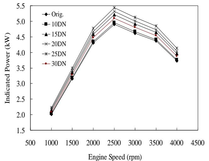
(b). Indicated power of new multi-degree hole injector nozzles
