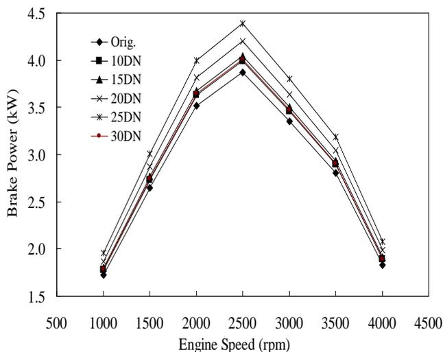
(b). Brake power of new multi-degree hole injector nozzles
