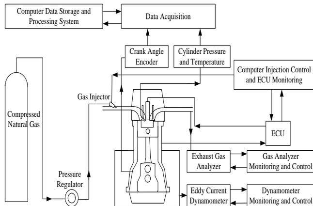
Figure 1: Schematic of CNG engine experimental testing
