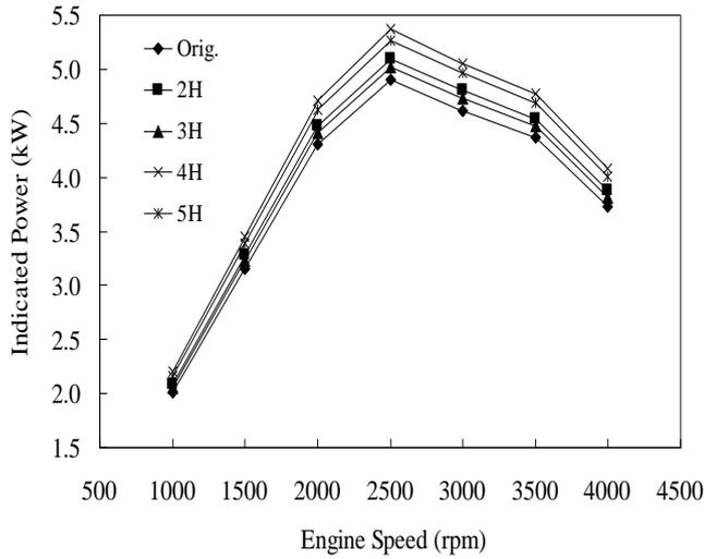
(d). Indicated power of new multi-hole injector nozzles
