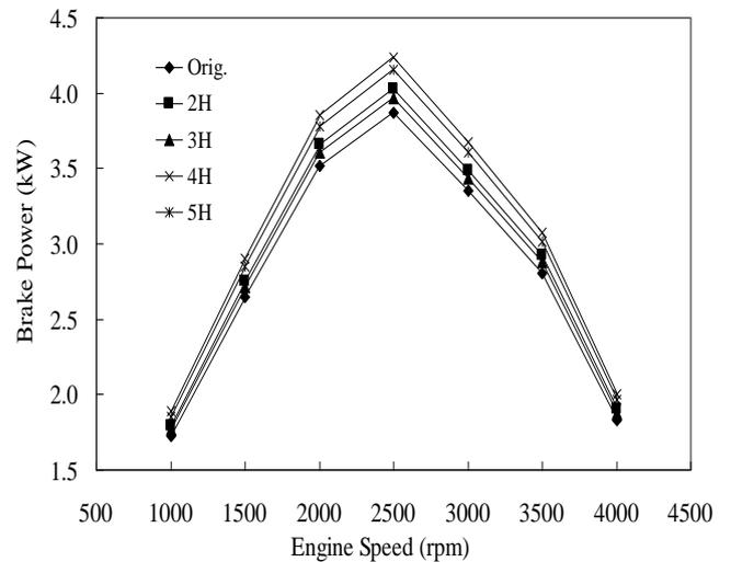
(d). Brake power of new multi-hole injector nozzles
