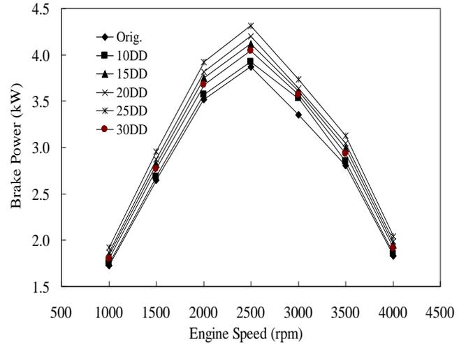
(c). Brake power of new multi-degree diffuser hole injector nozzles
