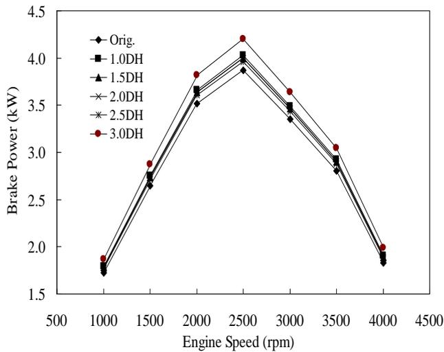
(a). Brake power of new multi-diameter hole injector nozzles
