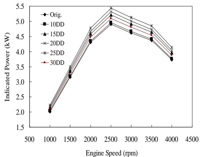
(c). Indicated power of new multi-degree diffuser hole injector nozzles
