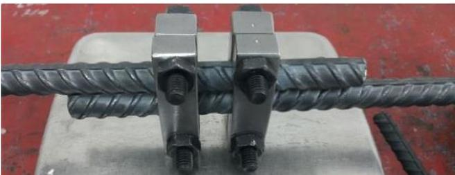
**Figure 13:** Installation of CT-1b on reinforcement D16
