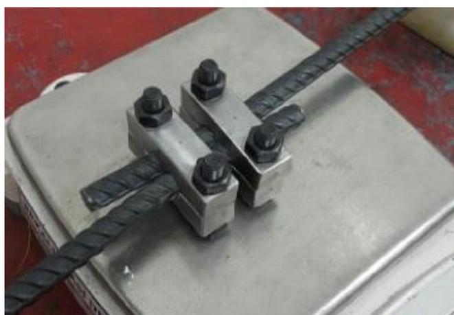
**Figure 15:** Damage patterns of the steel clamp
