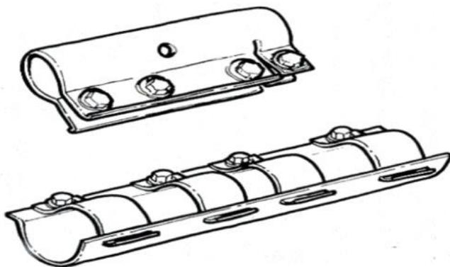
Figure 1: Solid-Type Steel Coupling Sleeve
