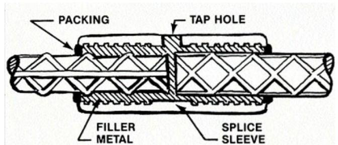
Figure 3: Steel-Filled Coupling Sleeve
