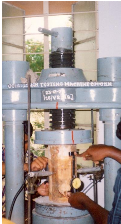
Figure 8: Concentric axial load test Corroded specimen
