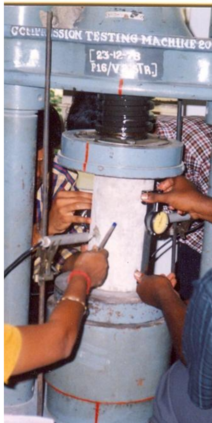
Figure 7: Concentric Axial Load Test Conventional Specimen
