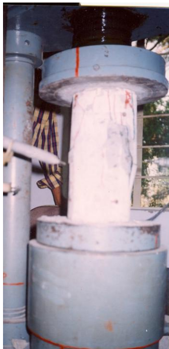
Figure 9: Failure mode of Conventional specimen
