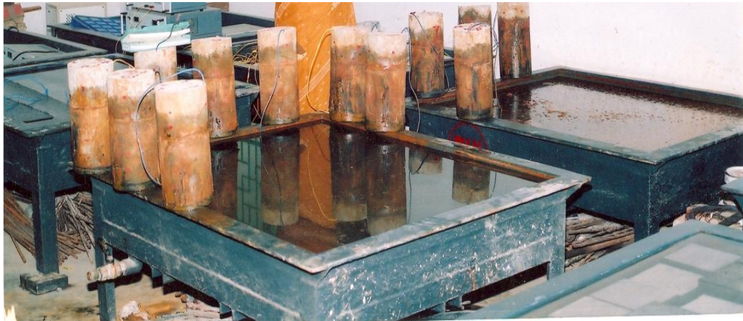
Figure 3: Scale Model Columns After The Accelerated Corrosion Process
