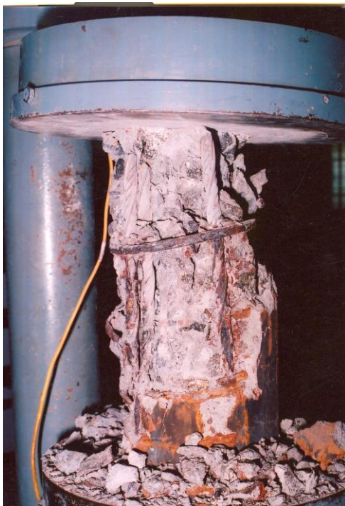
Figure 10: Views of failure of the specimen.
