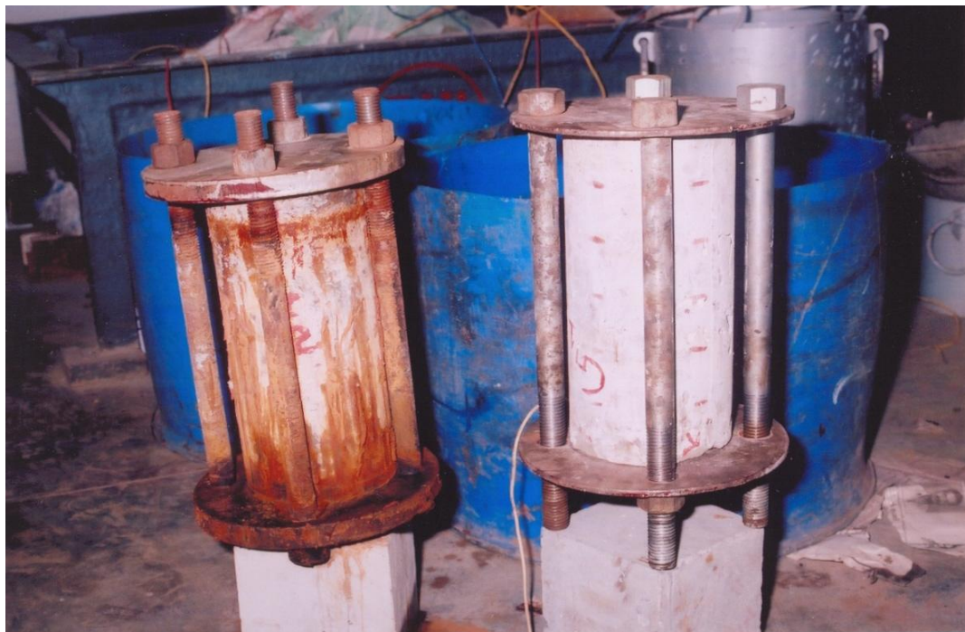
Figure 4: Scale Model Columns After The Accelerated Corrosion Process Under Loading Condition
