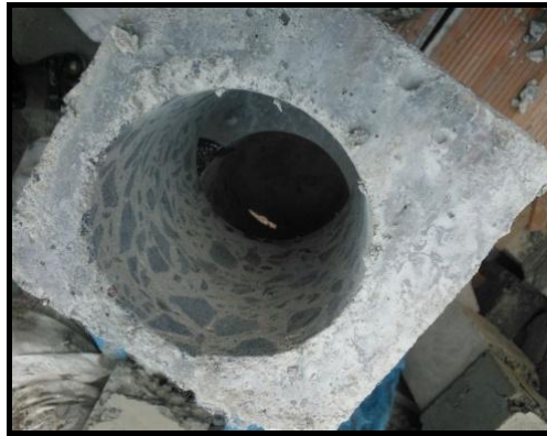
Figure 1: Cylindrical Core Extracted From Cube
