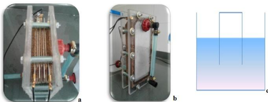
Fig.1. a) top view of electrolyzer, b) side view of electrolyzer and c) inverted beaker
