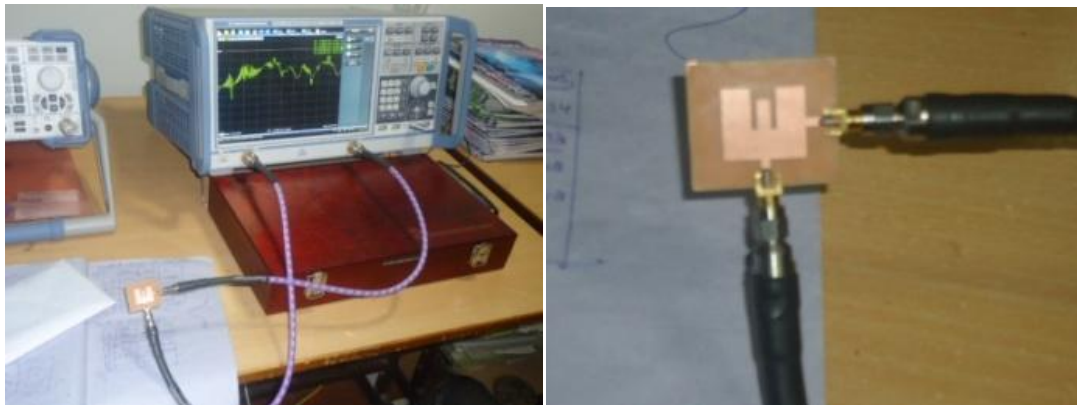
Fig. 13 Photo of fabricated antenna testing using Network analyser
