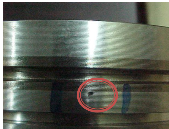
Fig.2 Insert blowhole is a casting defect – Seen as a small bubble like hole just below the Alfin insert or the machined surface of the piston.
