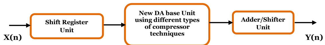
Fig.2. Block diagram of the proposed distributed arithmetic FIR Filter
