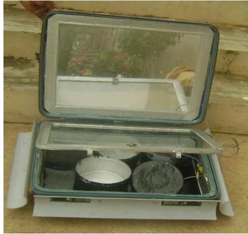
Fig.2. Photographic view of Aeroprofile Box Type Solar cooker
