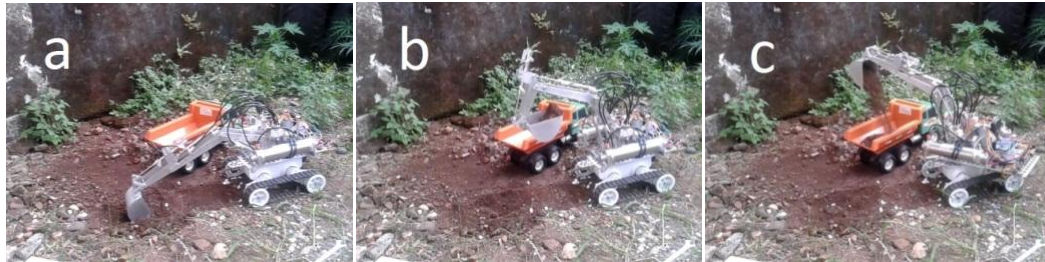
Figure18. Model of excavator fill the trucks model with soil material
