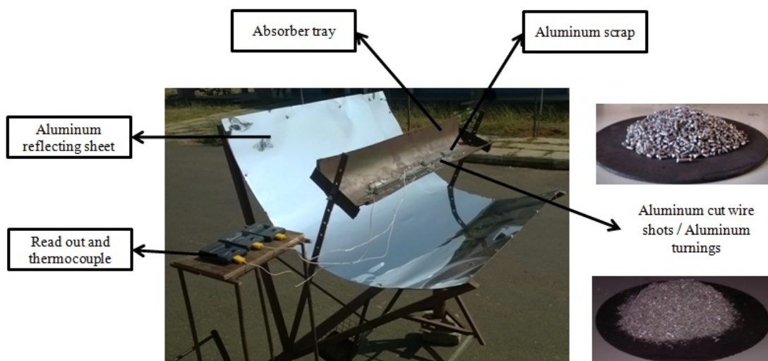
Fig. 2 Improved experimental setup with heat transfer enhancers
