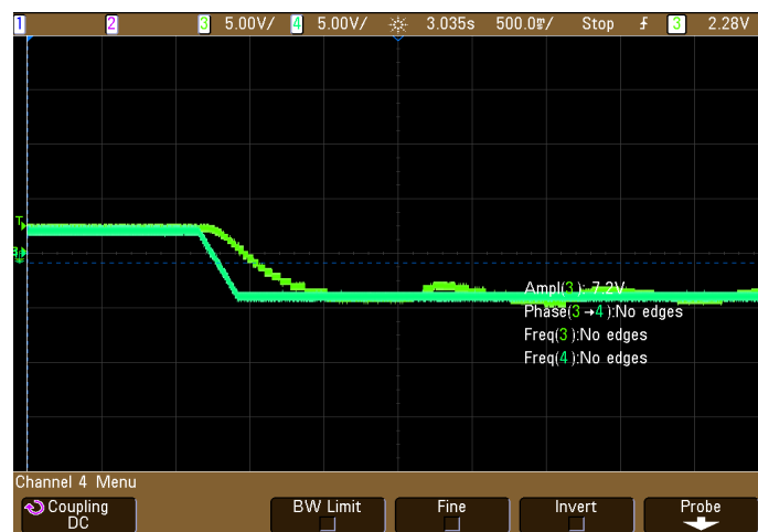
Figure 12: Speed control for step change 2500-500 rpm at 0.5kg
