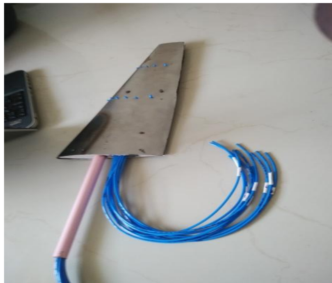
Figure 3 Fabricated wing structure without winglet (Flat)
