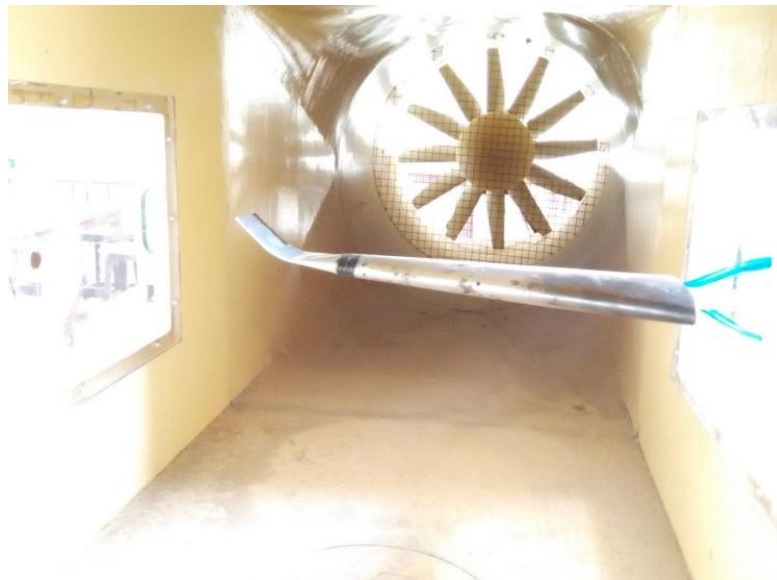
Figure 4 Experimental arrangement for testing with winglet of phase angle 25 deg.
