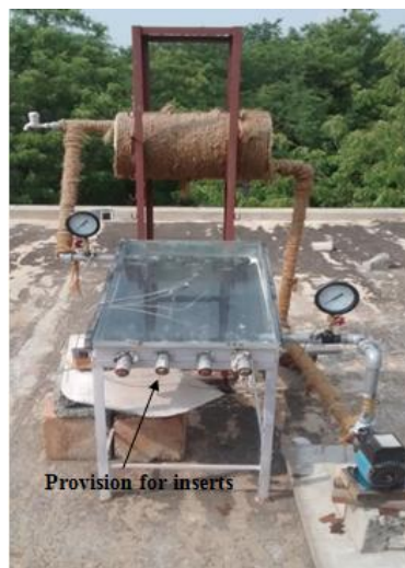
Figure 2 (b): Photographic view of modified solar water heater solar water heater
