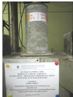
Figure 2: Proses Uji Tekan Sampel CTRB
