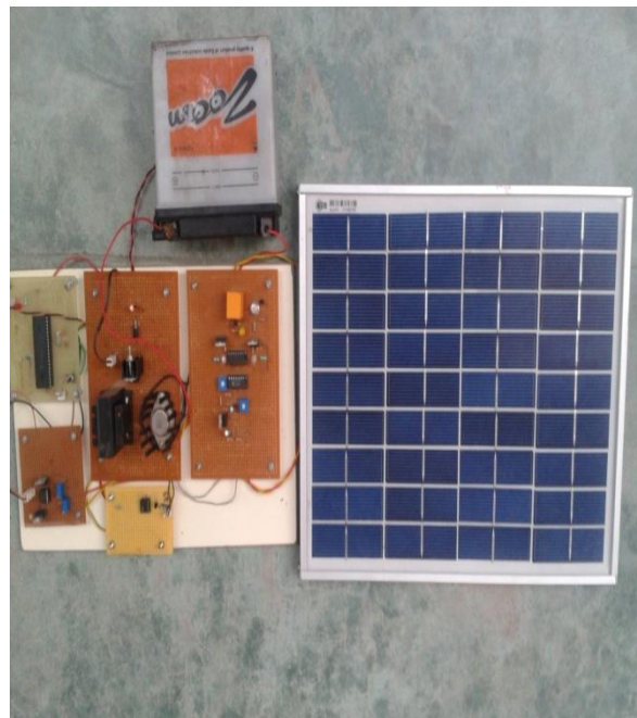
Figure 8: Testing of Circuit with Solar Panel
