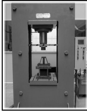
Figure 2. 200 ton Hydraulic press with clam assembly
