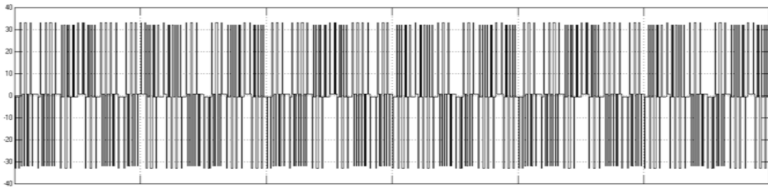
Figure 11(a): CMV waveform observed in 3 Phase 5 Level NPC Inverter operated with Multi Carrier PWM Technique without CMAF
