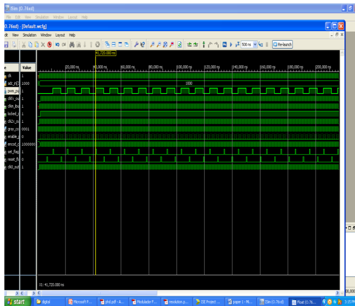
Figure 8: Simulation Waveform for duty cycle = 55.1% with adc:1000
