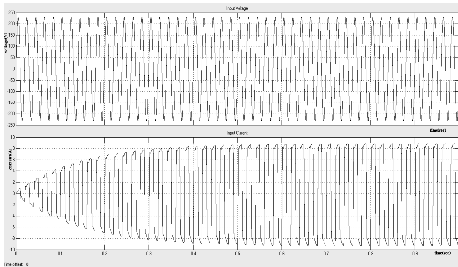
Figure 5c: Input voltage and Input current of conventional converter based SMPS
